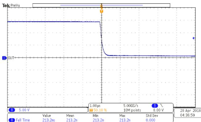
Figure 5. Critically Damped External Gate Resistor  $R_{GATE} = 7\text{-}\Omega$
