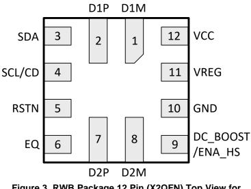
Figure 3. RWB Package 12 Pin (X2QFN) Top View for TUSB211, TUSB212, TUSB214 (no DC\_BOOST on TUSB211)
