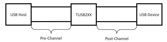
Figure 9. Pre-Channel and Post-Channel
