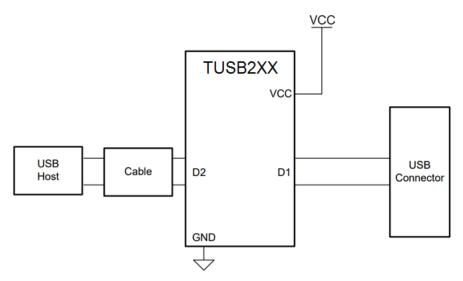
Figure 1. Simplified Schematic
