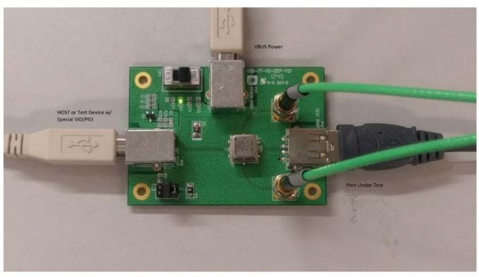
1. Use the USB-IF (Or Scope Vendor's) USB 2.0 Device High-Speed Test Fixture (See Figure 8). Connect the USB Test Fixture to the Head Unit USB Port to be tested.
