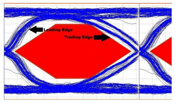
Figure 11. Leading and Trailing Edge
