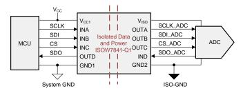
Figure 6. Integrated Isolated Power Supply for Isolated SPI
