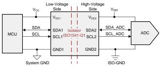
Figure 3. I2C Signals Isolated in Battery Management Systems
