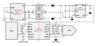
Figure 4. Discrete isolated Power Supply for Isolated SPI
