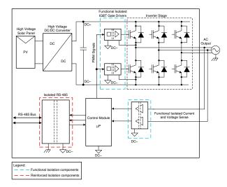
Figure 2. Solar Inverter Implementation
