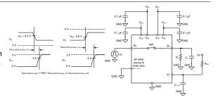
Figure 7-11. Fault Flag Recovery Time
