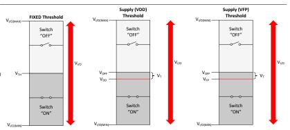
Figure 4-5. Overvoltage Protection
