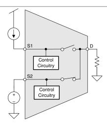
Figure 4-2. Injection Current Control
