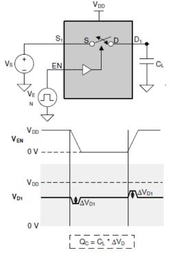
Figure 6-3. Charge Injection
