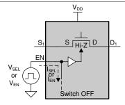
Figure 5-7. Control Input Leakage
