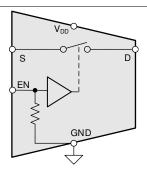
Figure 4-3. Integrated Pulldown Resistor on Logic Pin
