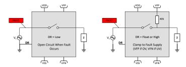
Figure 4-8. Drain Response Output
