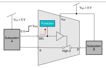
Figure 4-1. Fail-Safe Logic
