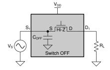
Figure 6-1. Source and Drain Off Capacitance
