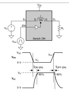
Figure 7-2. Device Turn on Time From Enable Pin
