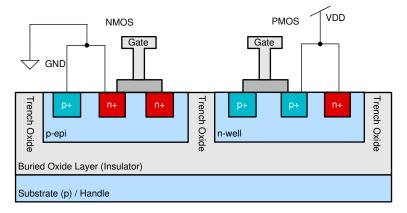
Figure 4-4. Latch-Up Immunity With SOI Process
