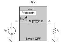
Figure 5-5. Powered-Off I/O Pin Leakage Current
