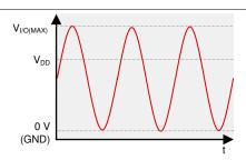
Figure 3-4. I/O Voltage Beyond Supply
