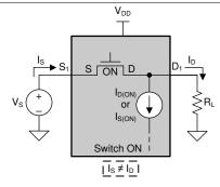
Figure 5-6. ON Leakage Current
