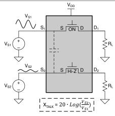
Figure 6-5. Channel-to-Channel Crosstalk
