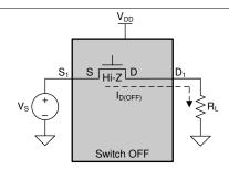
Figure 5-4. OFF Leakage Current
