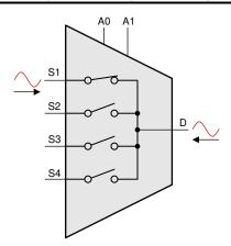
Figure 3-5. Bidirectional Signal Path
