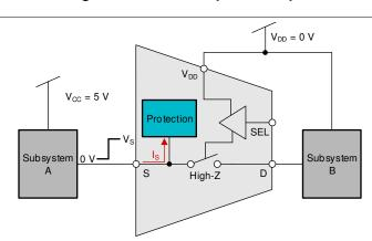
Figure 4-9. Powered-Off Protection
