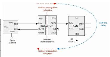
Figure 3. Total loop delay for isolated CAN system
