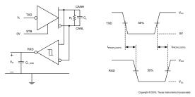
Figure 1. t<sub>PROP(LOOP)</sub>Test Circuit and Measurement
