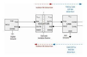
Figure 4. Total bit time for isolated CAN
