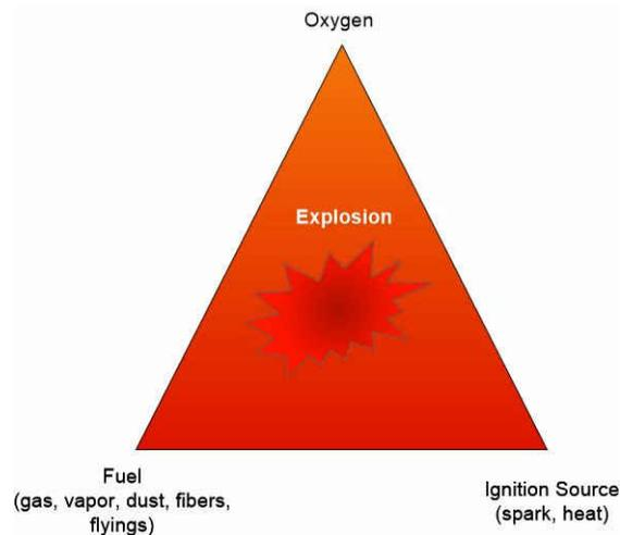
**Figure 1-1. Three Ingredients Forming the Explosion Triangle**
