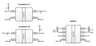
Figure 1. UART Optocoupler Circuit vs ISO6721 Digital Isolator Circuit
