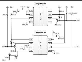
Figure 4. I2C Optocoupler Circuit
