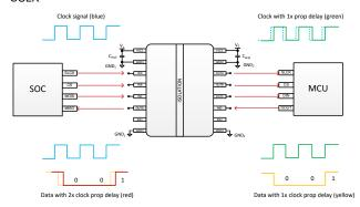
Figure 3. Digital Isolator Propagation Delay for SPI Loop Timing
