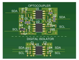
Figure 5. I2C Footprint of Optocoupler Circuit vs ISO1641 Isolator Circuit
