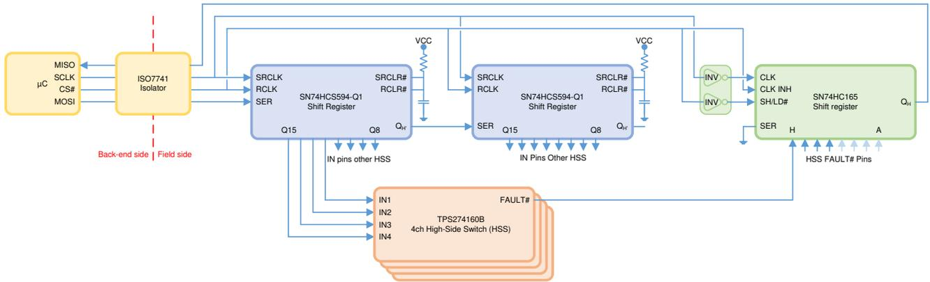
Figure 3. Block Diagram
