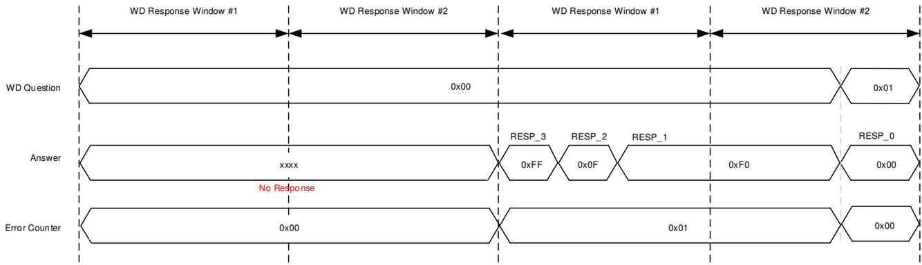
**Figure 7-5. Example of a Failed Cycle Due to the Controller Failing to Respond Before the End of the Timing Window**
