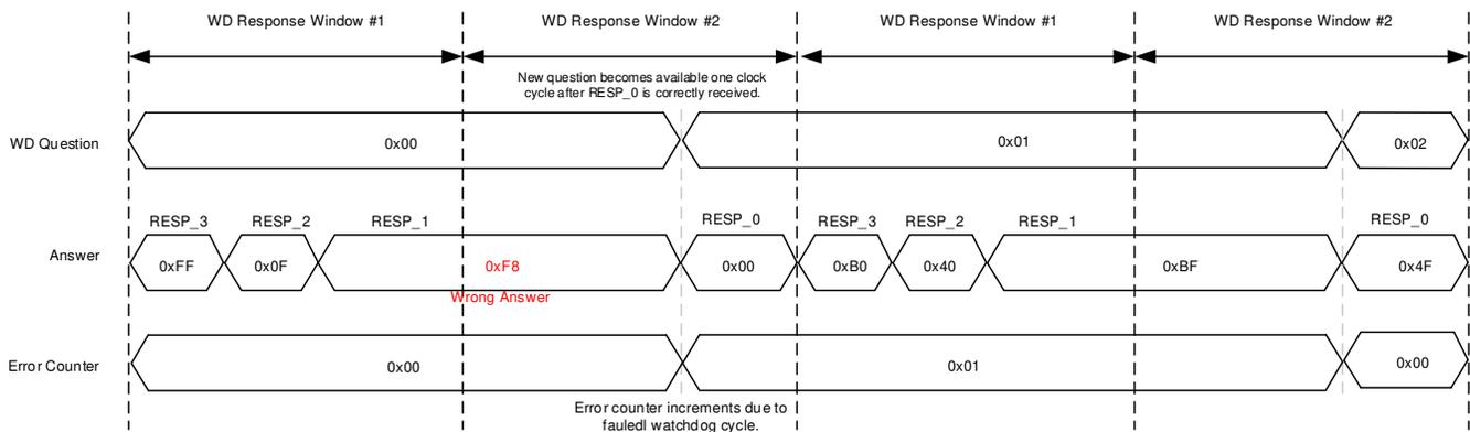
**Figure 7-3. Example of a Failed Cycle Due to an Incorrect Response**
