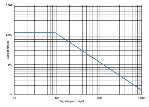
This system design uses a 1500-m cable. From the previous figure, the maximum recommended signal rate is 90kbps.
