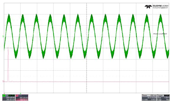
Figure 2-3. Phase current waveform and FFT - Continuous PWM modulation
