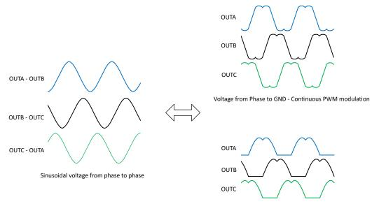
Voltage from Phase to GND - Discontinuous PWM modulation
