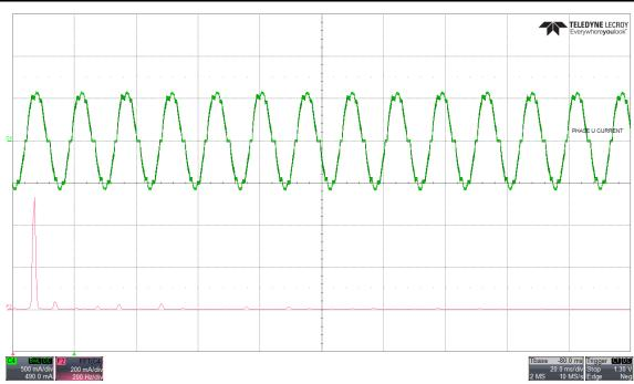
Figure 2-8. Phase current waveform and FFT - 150° Trapezoidal commutation
