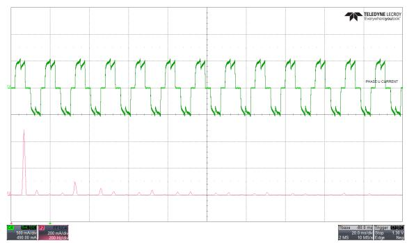
Figure 2-7. Phase current waveform and FFT - 120° Trapezoidal commutation
