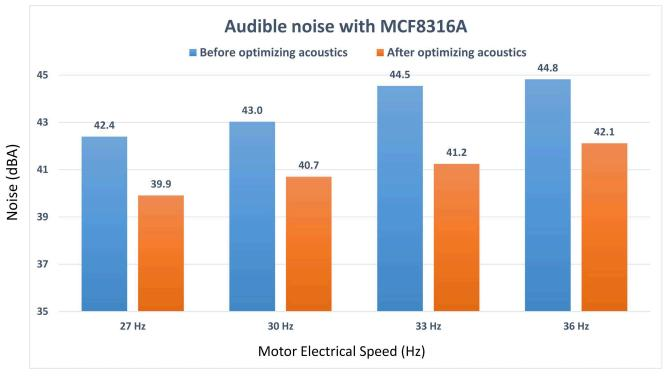
Figure 2-6. Audible Noise Comparison with MCF8316A
