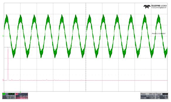
Figure 2-5. Phase current waveform and FFT - Dead time compensation enabled
