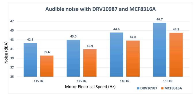
Figure 2-10. Audible noise comparison between MCF8316A and DRV10987
