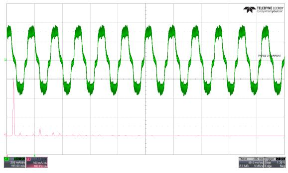
Figure 2-4. Phase current waveform and FFT - Dead time compensation disabled
