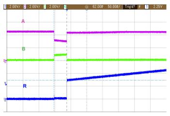
Figure 2-8. THVD1505 Powered Up with Mis-wiring and Driver On
