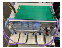
Figure 1-3. FR4 board with SMA connectors
