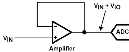
**Figure 20. Input Offset Voltage ( $V_{IO}$ )**
