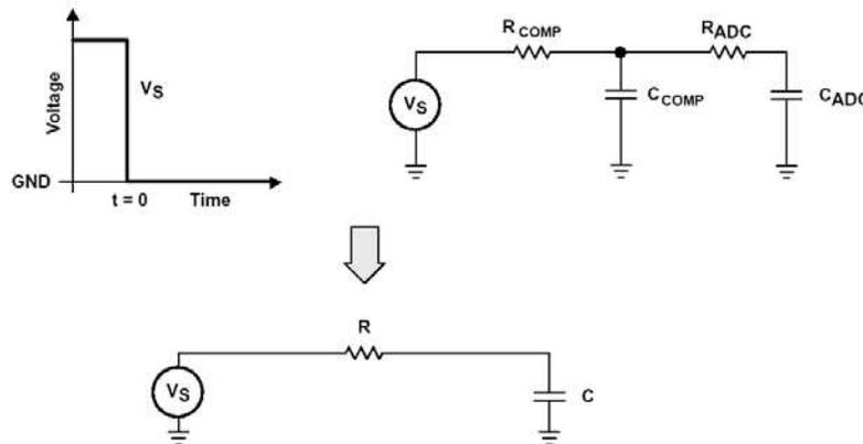
**Figure 17. Circuit Simplification**
