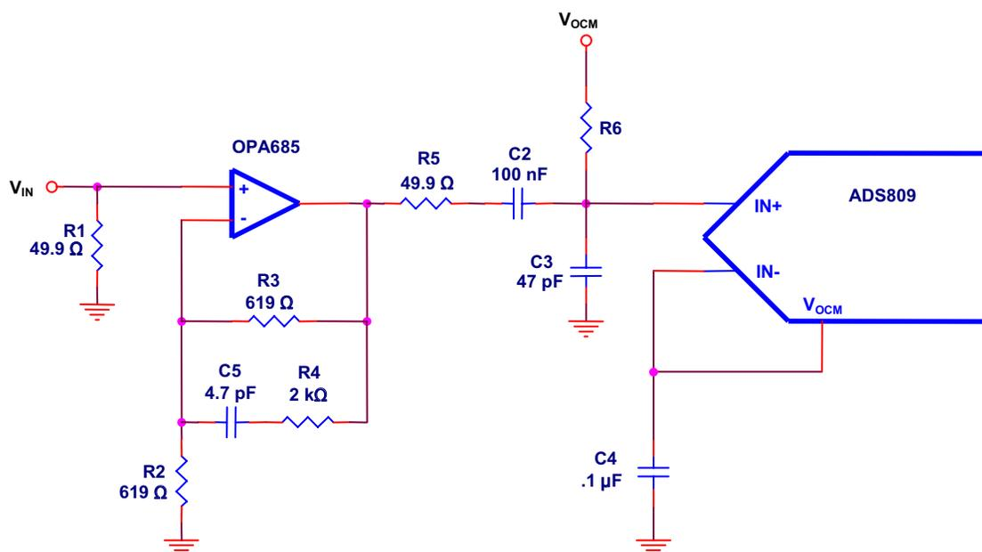
**Figure 21. Example of Buffer Operational Amplifier Design**
