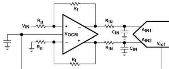
Figure 16. Fully Differential Input to the ADC
