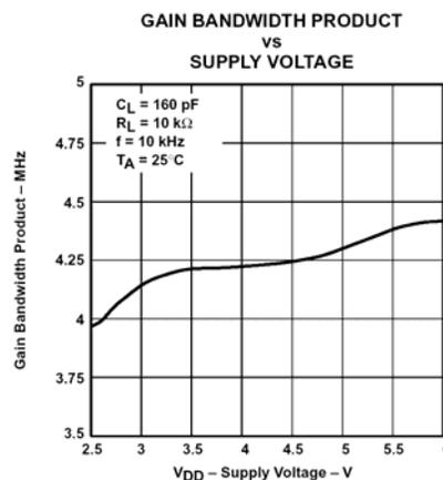
**Figure 9. Typical Gain Bandwidth Product Graph (TLV2460)**
