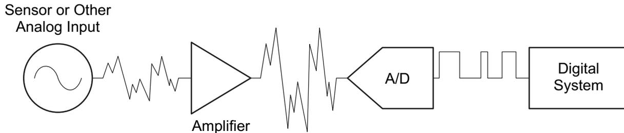
**Figure 1. Amplifier and ADC**
