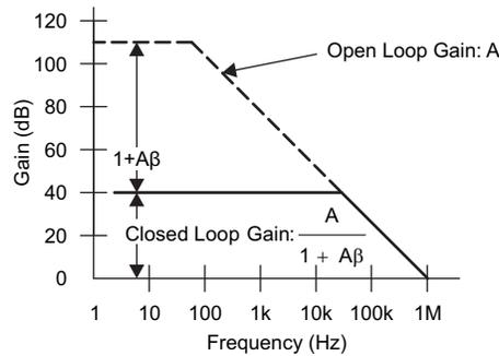
Figure 3. Closed Loop Bode Plot
