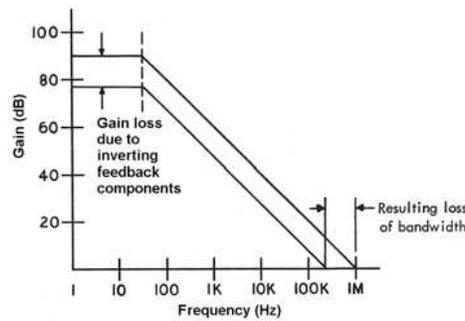
**Figure 7. Effect of Inverting Stage Components on Gain**
