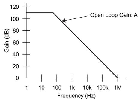
**Figure 2. Open Loop Bode Plot of an Operational Amplifier**
