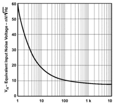
**Figure 11. Noise Characteristic of a Typical Operational Amplifier**
