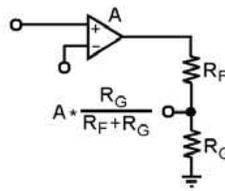
**Figure 5. Noninverting Stage With Loop Broken**
