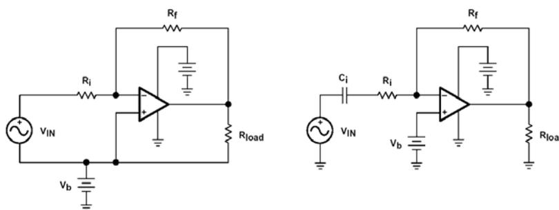
Figure 19. Input Signal Biasing Circuits
