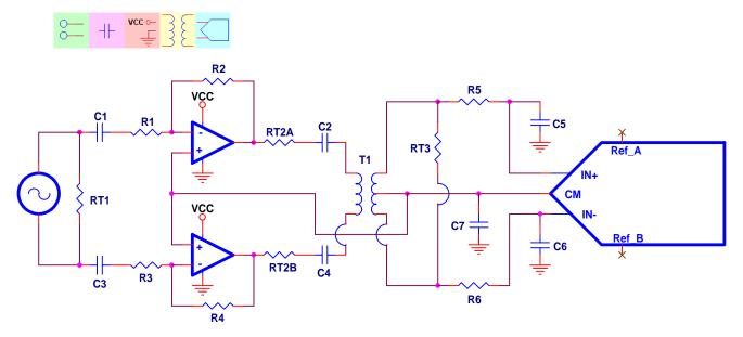
Figure 30. Differential Input, AC-Coupled, Single Supply
