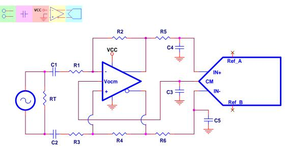
Figure 6. Differential Input, AC-Coupled, Single Supply
