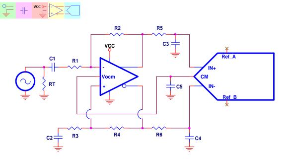
Figure 3. Single-Ended Input, AC-Coupled, Single Supply
