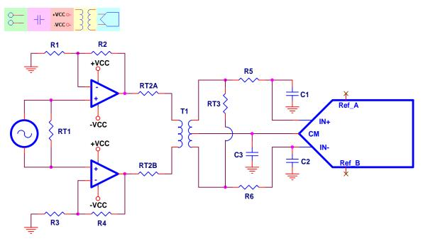
Figure 31. Differential Input, AC-Coupled, Dual Supply
