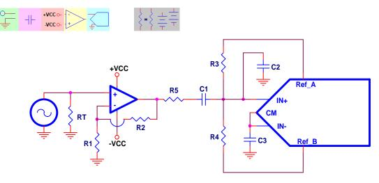
Figure 13. Single-Ended Output, Single-Ended Input, AC-Coupled, Dual Supply
