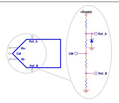
Figure 2. Reference Structure of Common ADCs
