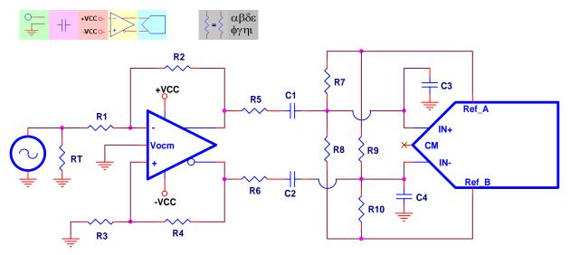
Figure 4. Single Ended Input, AC-Coupled, Dual Supply
