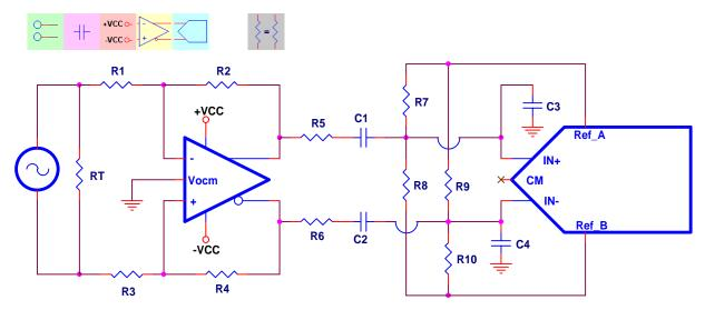
Figure 7. Differential Input, AC-Coupled, Dual Supply
