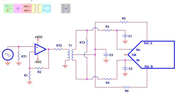
Figure 29. Single-Ended Input, AC-Coupled, Dual Supply
