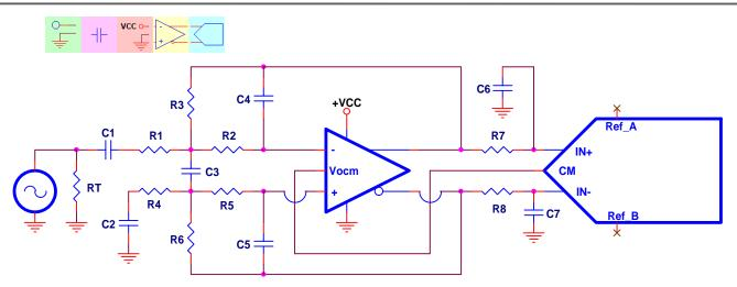
Figure 10. Antialias Filter Using a Fully Differential Op Amp
