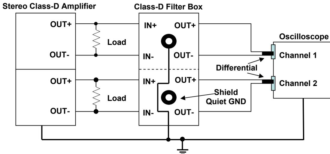
**Figure 4. Stereo Class-D Amplifier and RC Filter Box for Output Power Measurement**
