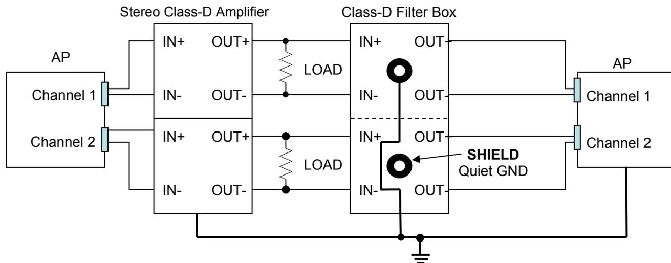
**Figure 5. Stereo Class-D Amplifier and RC Filter Box for THD+N Measurement**
