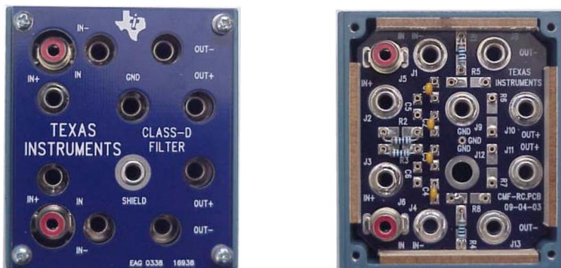
**Figure 3. Top and Inside View of Texas Instruments RC Filter Box**
