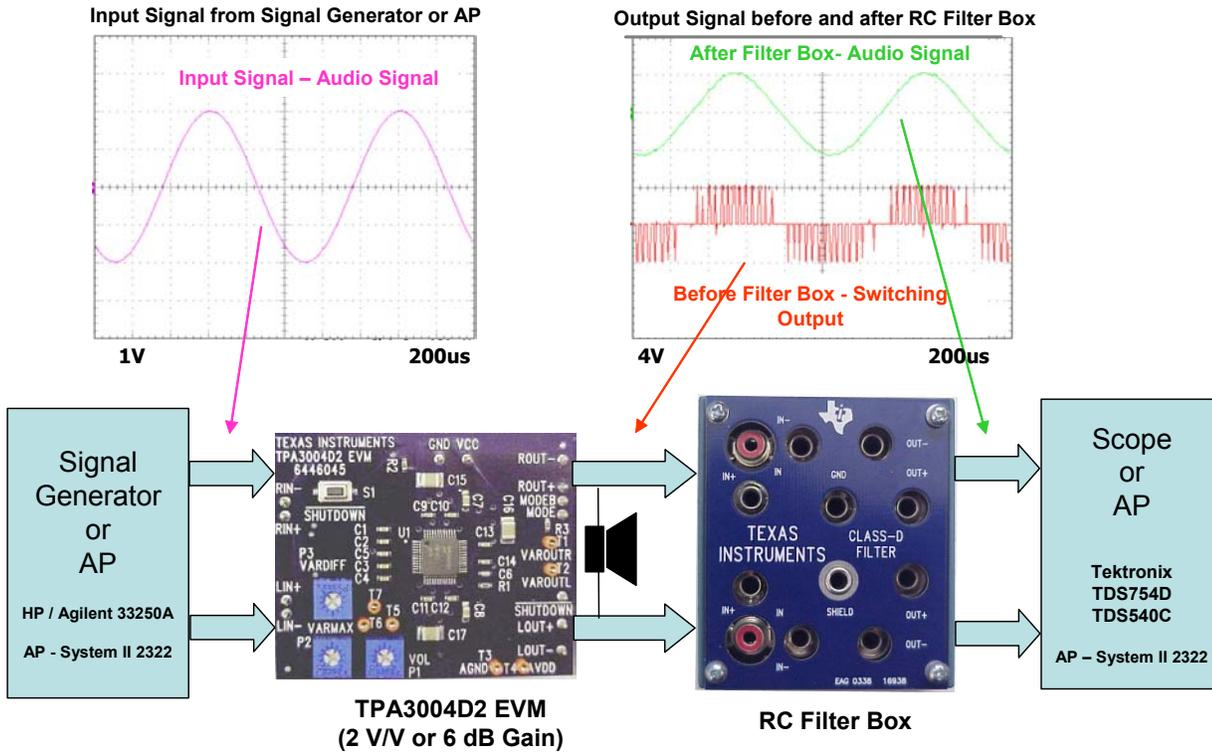
Figure 1. Filter Box Setup for Output Power Measurement
