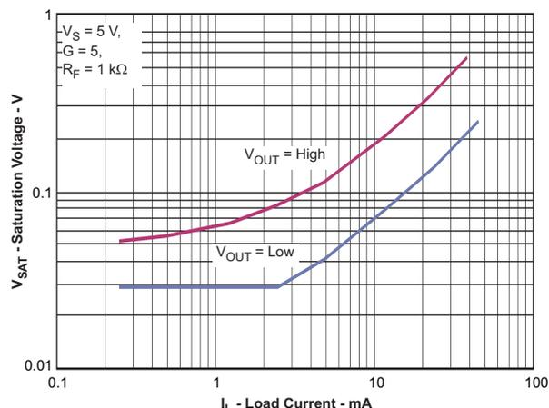
Figure 12. Output Saturation Voltage vs Load Current
