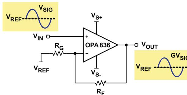
Figure 1. Non-Inverting Amplifier
