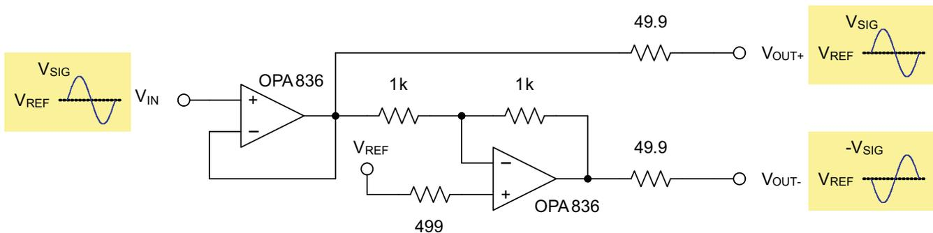
Figure 4. CAT 5 Line Driver with Gain = 2 V/V (6 dB)
