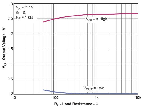
Figure 9. Output Voltage Swing vs Load Resistance
