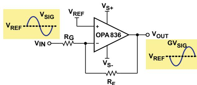
Figure 2. Inverting Amplifier
