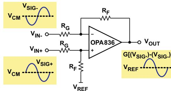
Figure 5. Differential to Single Ended Amplifier
