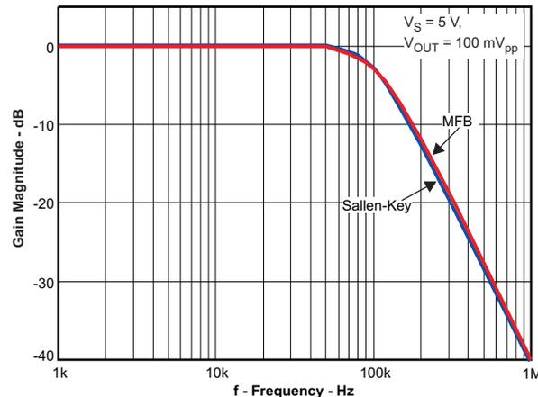
**Figure 28. MFB and Sallen-Key 2<sup>nd</sup> Order Low-Pass Butterworth Filter Response**
