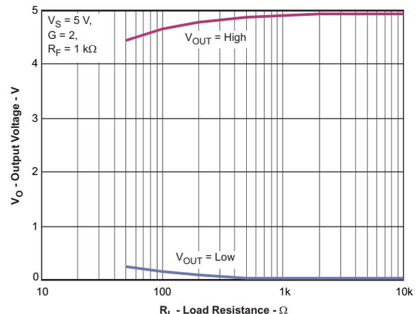
Figure 10. Output Voltage Swing vs Load Resistance
