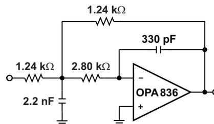
Figure 26. MFB 100kHz 2<sup>nd</sup> Order Low-Pass Butterworth Filter Circuit
