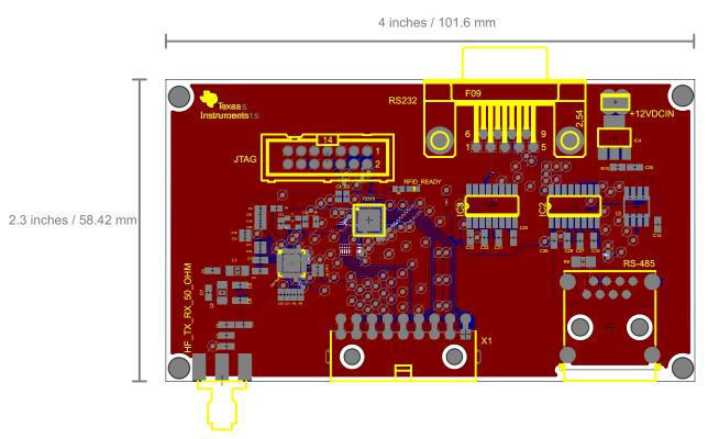
Figure 13. RFID Controller Board Layout
