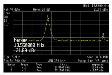
Figure 9. TRF7960A to PE42440 to PE4257 out (Approximately 0.8-dBm Loss)
