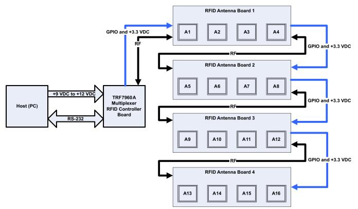
Figure 1. TRF7960A Multiplexer RFID System Block Diagram
