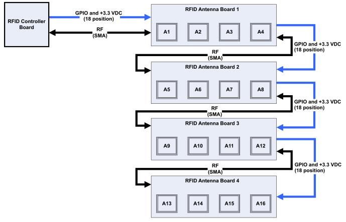
Figure 15. Signal Cascade Concept
