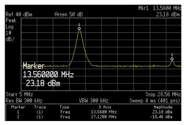
Figure 7. TRF7960A Out (Approximately +23 dBm)
