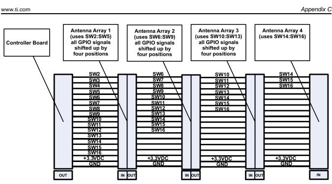
Figure 16. Cabling for Signal Cascade Concept
