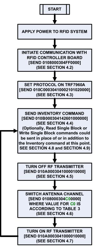
Figure 6. Example Application Flow Chart
