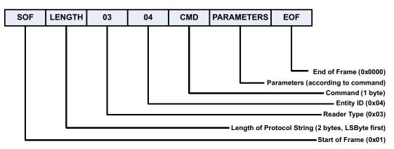
Figure 5. RFID Controller Host Protocol General Format
