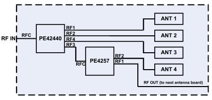
Figure 4. PE42440 and PE4257 Antenna Circuit Arrangement Detail Diagram
