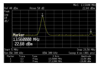
Figure 8. TRF7960A to PE42440 Out (Approximately 0.5-dBm Loss)
