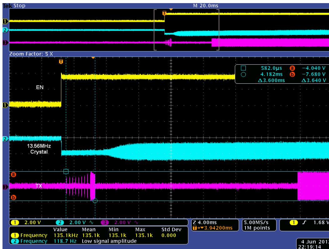
Figure 1. TX Out Behavior When EN is Line Raised (Register 0x0B left at default)
