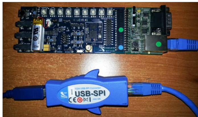
Figure 2. CSR Programming Setup
