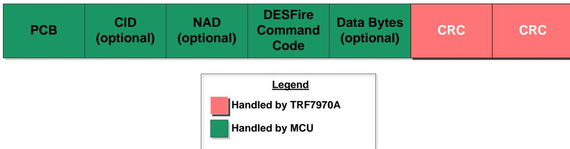
**Figure 3. Frame Format for Data Exchange Commands Using DESFire APDUs**
