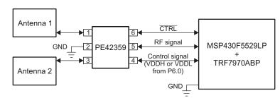
NOTE: The inverse signal of CTRL is supplied to pin 6.
