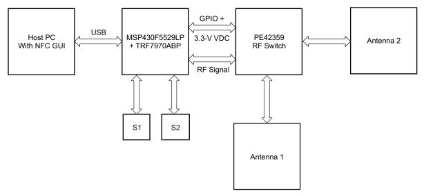
Figure 1. Block Diagram of Reader Antenna Multiplexing Demo
