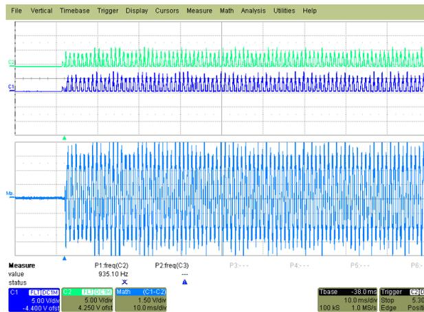
Figure 22. Volume Ramp Rate Control Disabled
