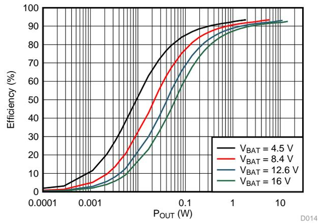
Figure 4. Output Efficiency, R<sub>L</sub> = 8 Ω, F<sub>s</sub> = 1 kHz
