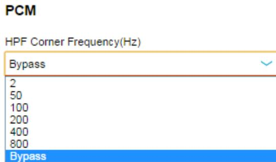
Figure 29. High-Pass Filter Configuration
