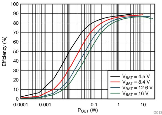
Figure 3. Output Efficiency, R<sub>L</sub> = 4 Ω, F<sub>s</sub> = 1 kHz
