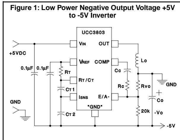
With this arrangement, the inductor (L) charges when the IC output is high and discharges or flies-back when the IC output goes low. Energy stored during the inductors charging time is transferred to the output capacitor (Cout) during the flyback, or OFF portion of the cycle. When a BiCMOS PWM control IC is used, the external diode can be replaced by the MOS channel and body diode of the
