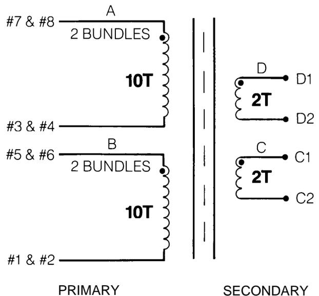
Figure 5. Transformer Schematic
