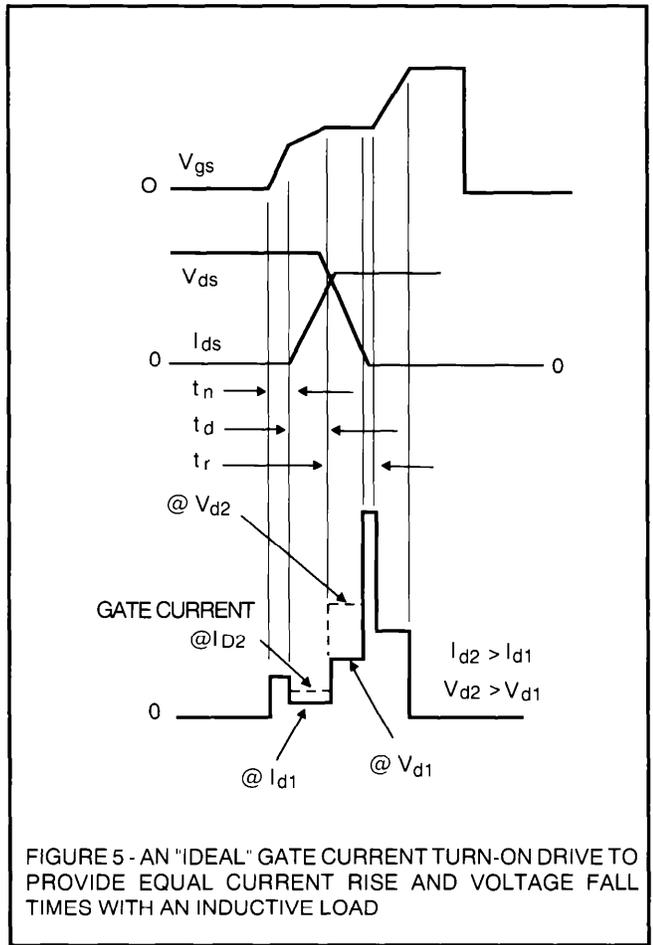
FIGURE 5 - AN "IDEAL" GATE CURRENT TURN-ON DRIVE TO PROVIDE EQUAL CURRENT RISE AND VOLTAGE FALL TIMES WITH AN INDUCTIVE LOAD
