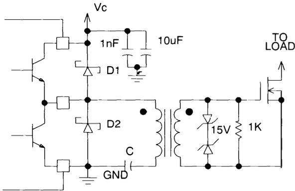
D1,D2:UC3611 SCHOTTKY DIODE ARRAY
