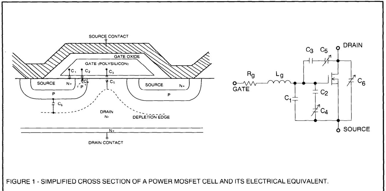
FIGURE 1 - SIMPLIFIED CROSS SECTION OF A POWER MOSFET CELL AND ITS ELECTRICAL EQUIVALENT.
