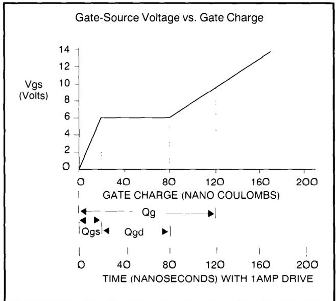
**First of all, and most importantly, the average capacitive load represented by the FET to the IC driver is NOT the specified MOSFET input capacitance, Ciss. The effective input capacitance, Ceff, is the total charge divided by the final gate voltage, Vgs(f);**
