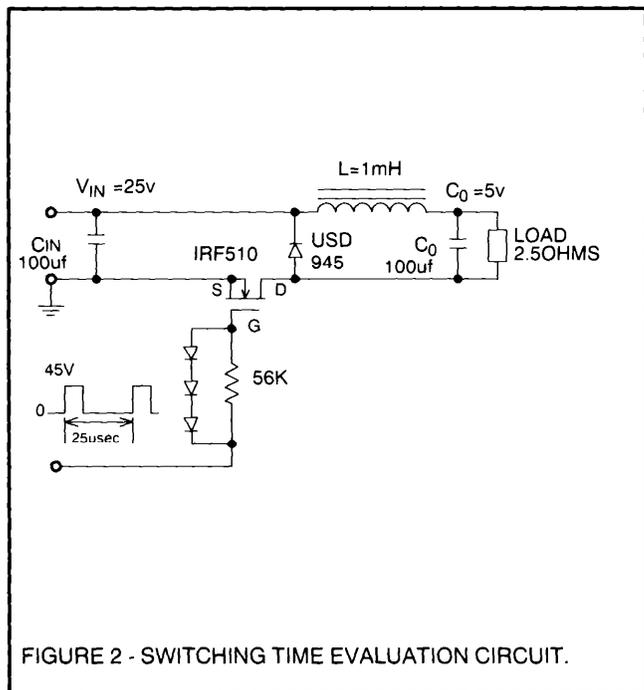
FIGURE 2 - SWITCHING TIME EVALUATION CIRCUIT.
