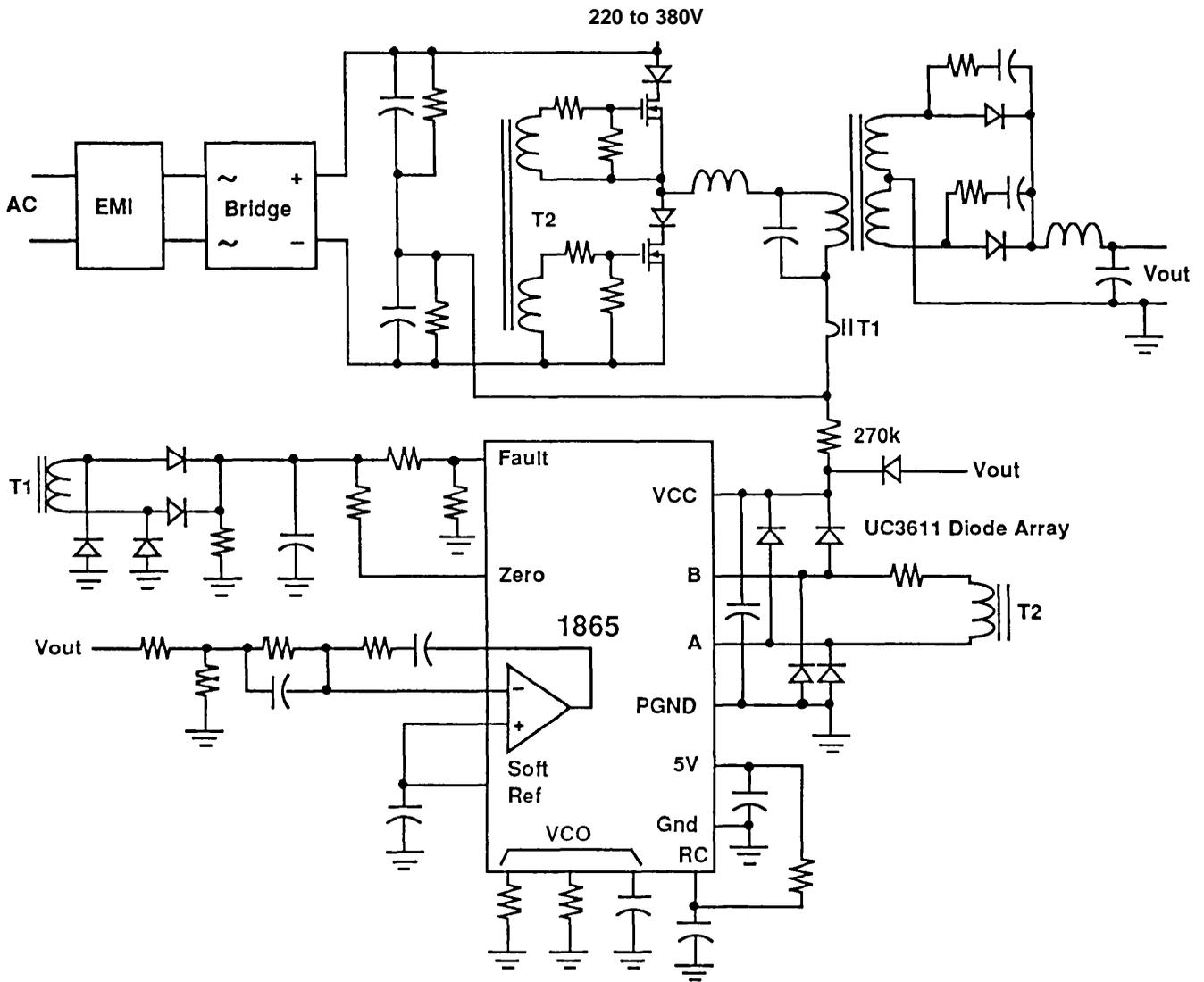
Figure 15. ZCS Off-Line Half-Bridge Converter With UC1865
