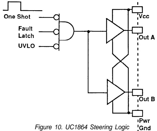
Figure 10. UC1864 Steering Logic
