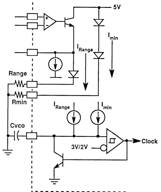
Figure 3. Error Amplifier and Voltage Controlled Oscillator
