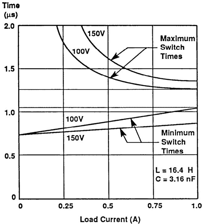
Figure 6. Minimum/Maximum Switch Time vs Load Current
