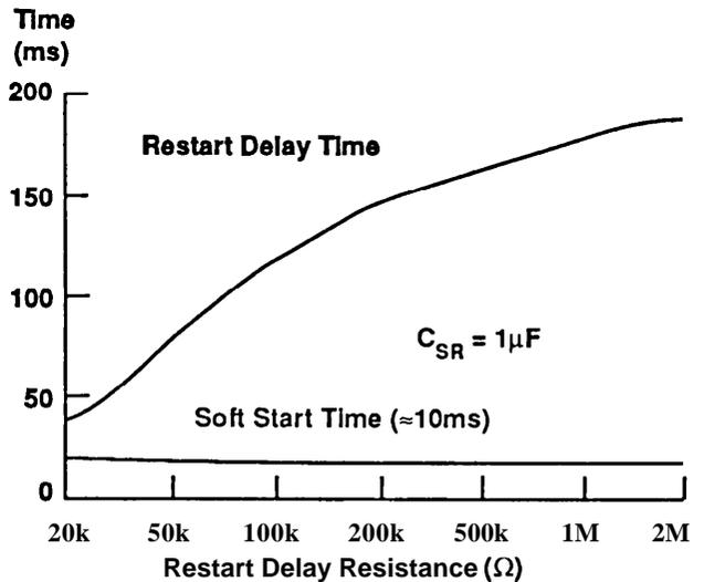
Figure 13. Soft Start And Restart Delay Times
