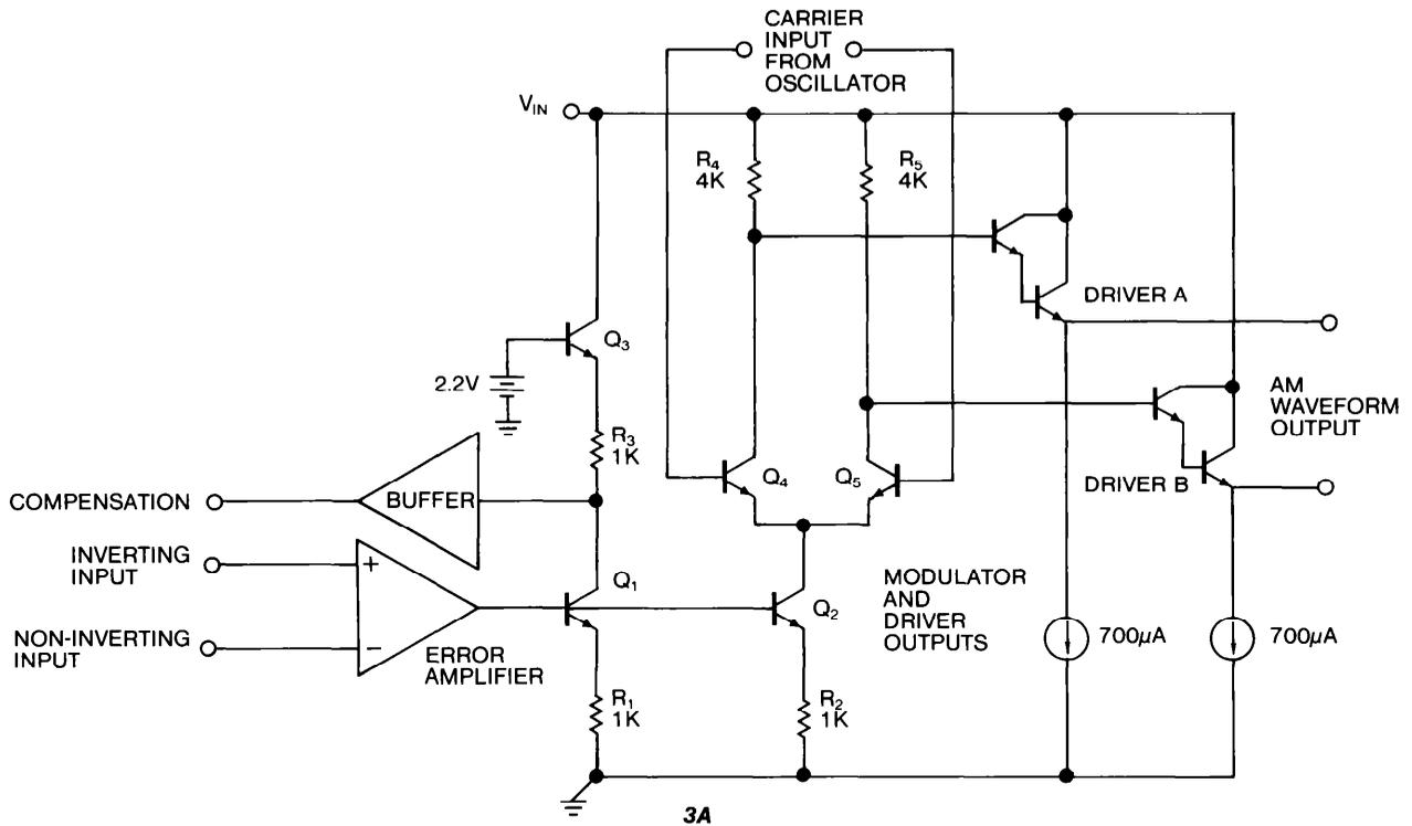
**FIGURE 3: The Compensation Output on the UC7907 can be used to Accurately Control the AM Waveform Output. A Simplified Schematic, (a) Shows the internal Signal Split into the Modulator: Voltage Waveforms, (b) Across the Modulator Outputs, and at the Compensation Output show the Modulator Transfer Characteristic.**
