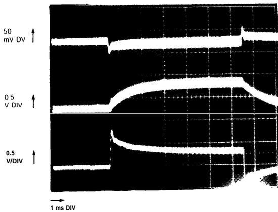
**FIGURE 11: The Transient Response of the 5V Output (Top Trace), to a 3.0A Step Load Change Reflects the Extended Bandwidth of the 5V Loop. The Open-Loop 12V Output (Middle), Responds to the Effects of Cross Regulation. The Feedback Error Signal (Lower) Coupled Through the UC1901 is Measured at the UC1840 Error Amp. Output.**
