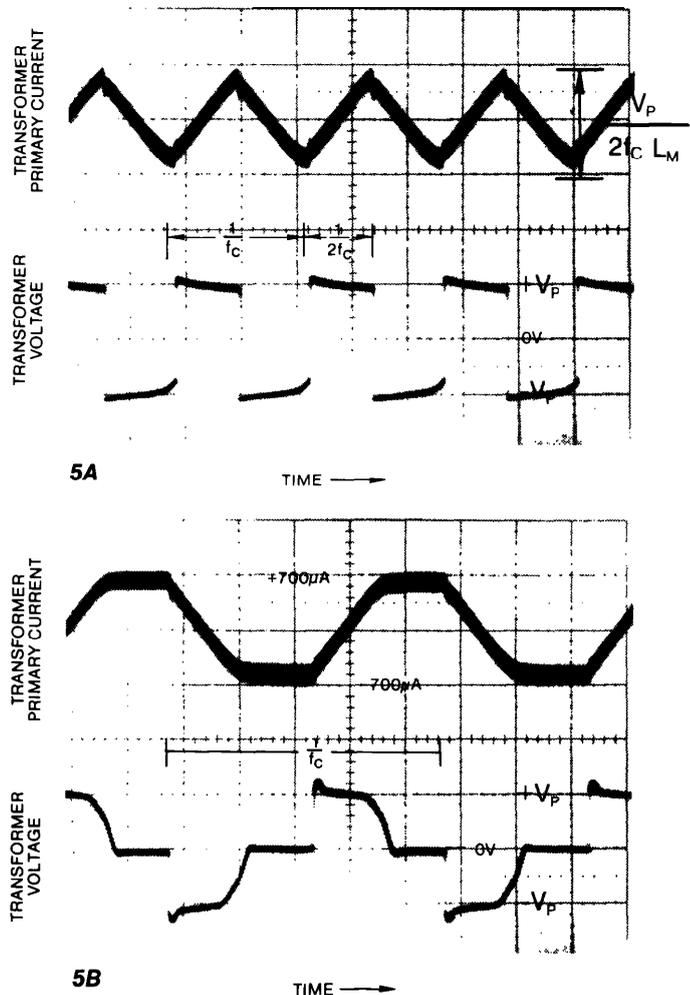
**FIGURE 5:** The UC1901 Driver Outputs Follow the Modulator Output Square Wave, (a.), Sourcing and Sinking Current Levels Dependent on Transformer Inductance, Carrier Frequency, and Voltage Level. When the Bias Level of the Driver Outputs,  $I_P$ , is Reached, (b.), a Tri-state Waveform is Coupled Across the Transformer; the Peak Voltage Level Though, Remains Approximately the Same. The Reflected Load Currents are Assumed Negligible.
