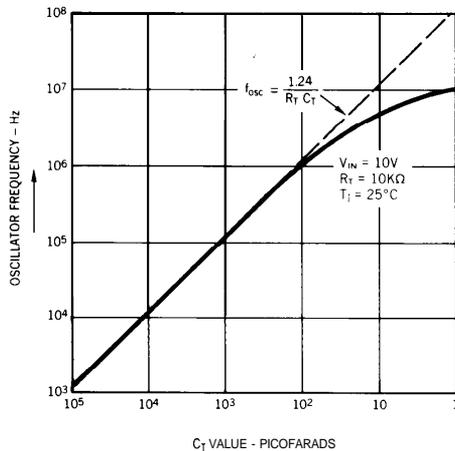
**FIGURE 7: UC1901 Oscillator Frequency.**
