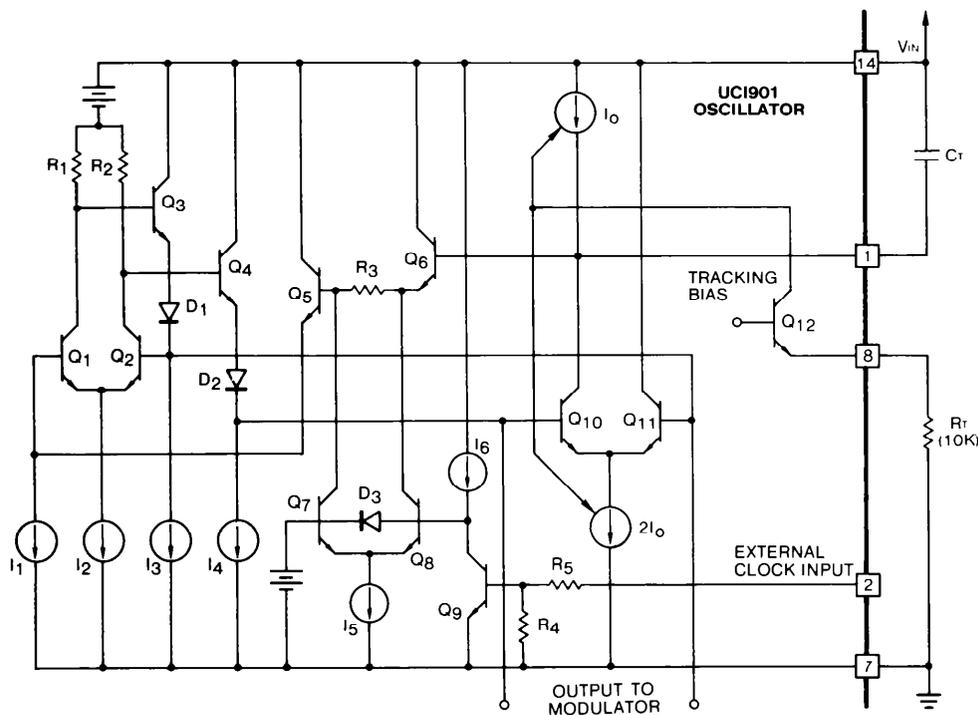
FIGURE 6: UC1901 High Frequency Oscillator Simplified Schematic.
