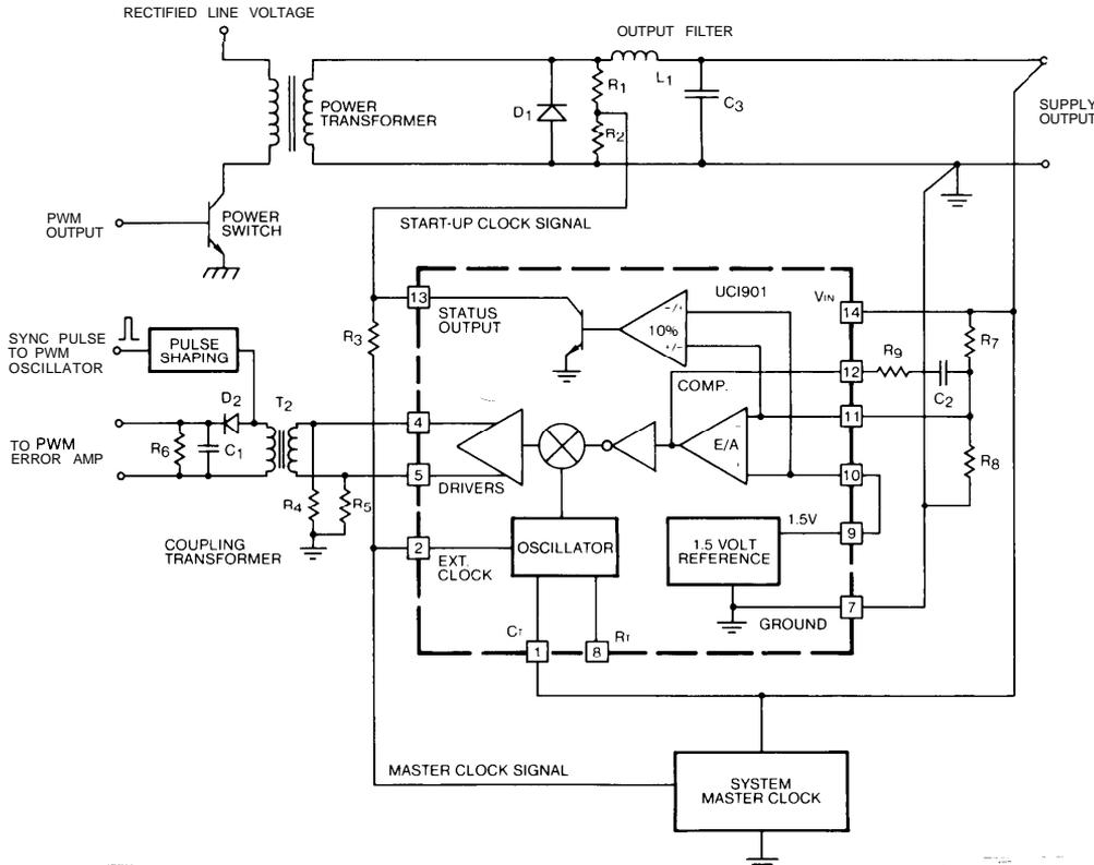
**FIGURE 8: The Status Output on the UC1901 is used in the Start-Up of a Power Supply Synchronized to a Secondary Referenced Master Clock. The Coupling Transformer Carries the Feedback and Clock Signals. The Status Output is used to Sequence Clock Signals to the UC1901 External Clock Input During Start-Up.**
