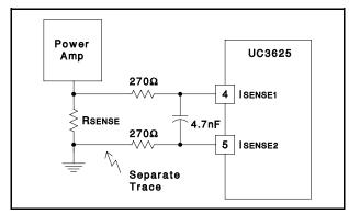
Figure 4: Proper Current Sense Layout
