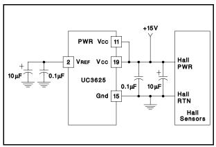
Figure 1: Recommended Power Connections and Decoupling
