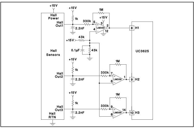
Figure 3: Comparator Sense of Hall Sensors
