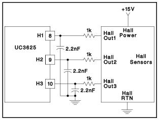
Figure 2: Recommended Hall Filtering
