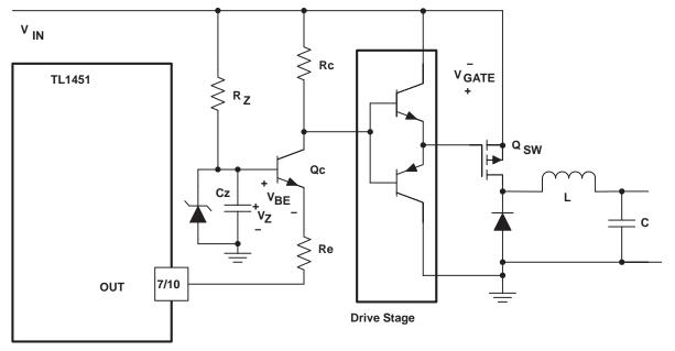
Figure 2. TL1451 With Cascode Transistor
