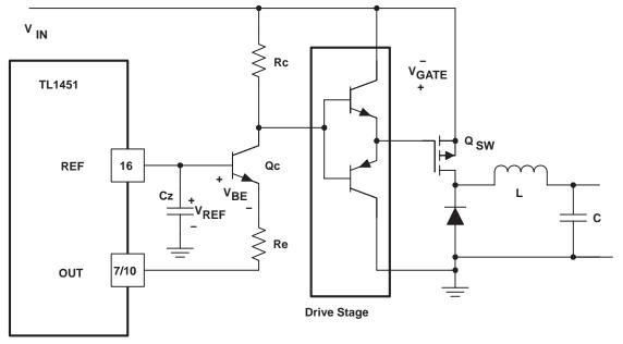
Figure 3. TL1451 With Cascode Using V<sub>REF</sub> Base Drive
