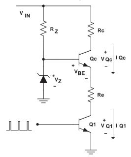
Figure 1. An NPN Transistor With Cascode
