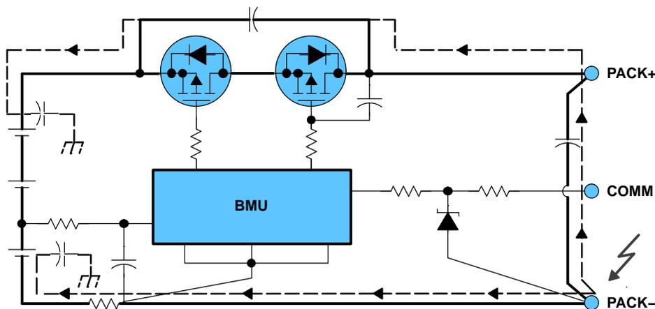
Figure 3. ESD Hit to PACK- Connector Pin
