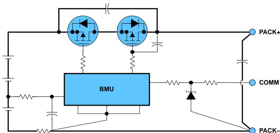
Figure 1. Basic Battery Pack Block Diagram
