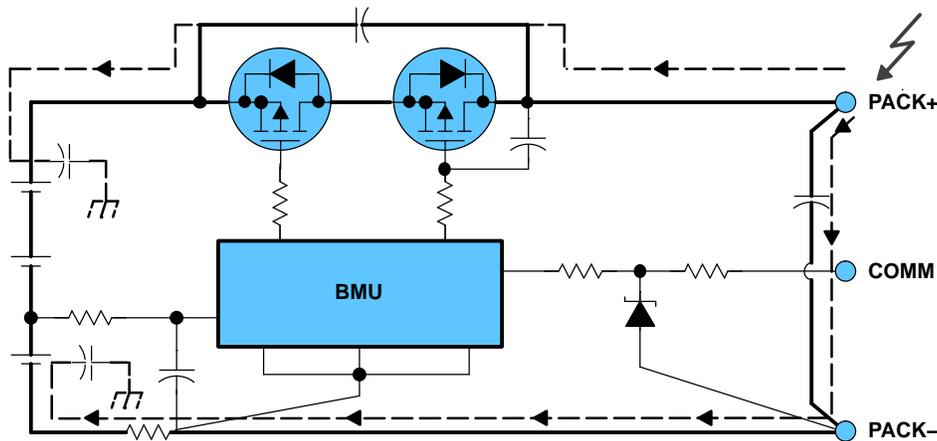
Figure 2. ESD Hit to PACK+ Connector Pin
