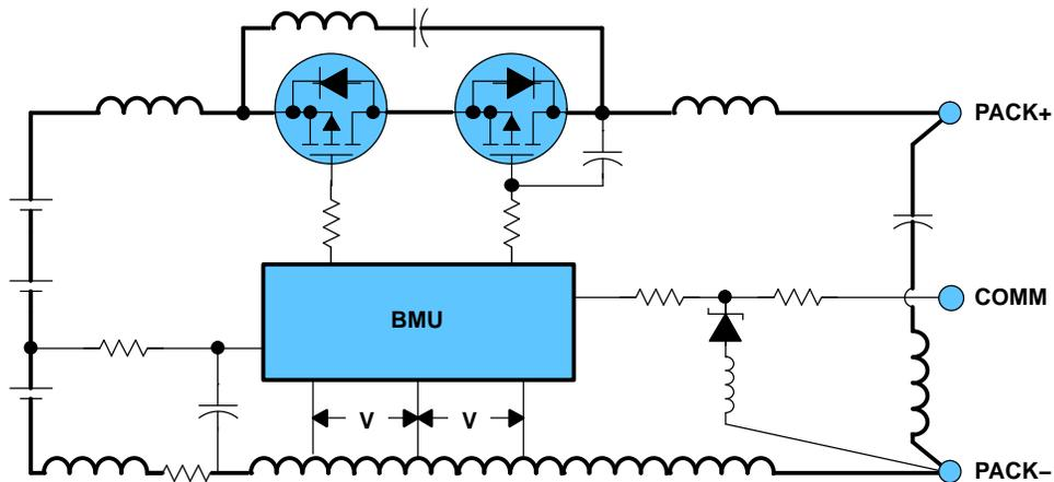
Figure 7. BMU Electronics Can Be Disrupted and Damaged From Circulating Ground Currents
