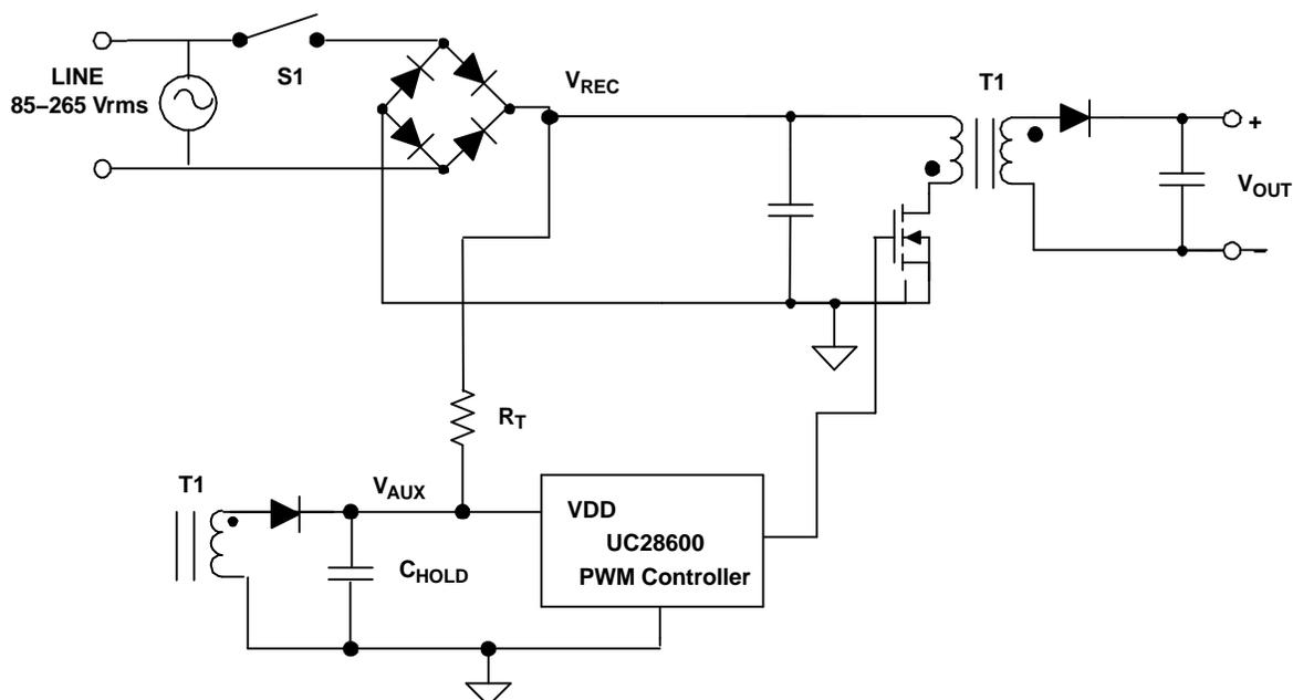
Figure 1. Offline Power Supply with Traditional Bootstrap Startup
