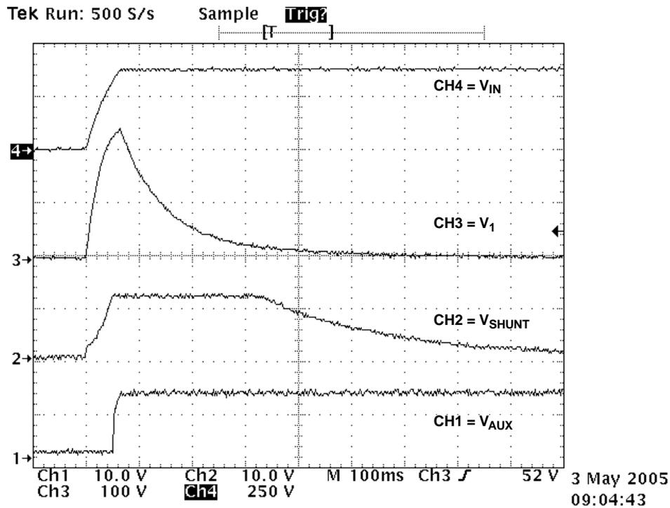
Figure 4. Startup with 375 V DC Applied to the Input.
