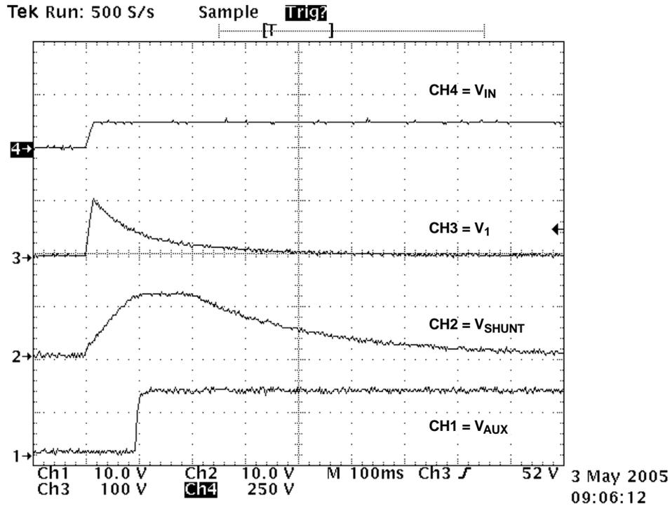
Figure 3. Startup with 120 V DC Applied to the Input.
