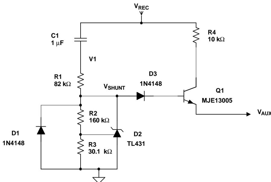
**Figure 2. Low Power Standby Bootstrap Circuitry**
