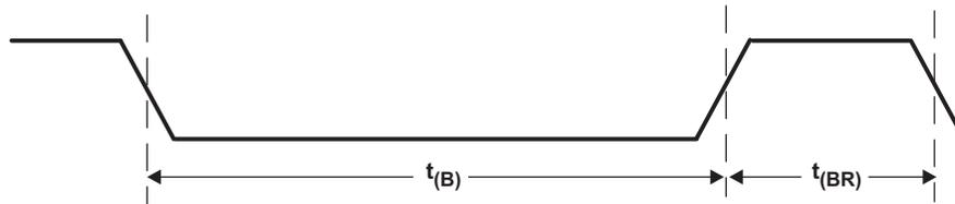
**Figure 2. HDQ Break and Break Recovery Timing**
