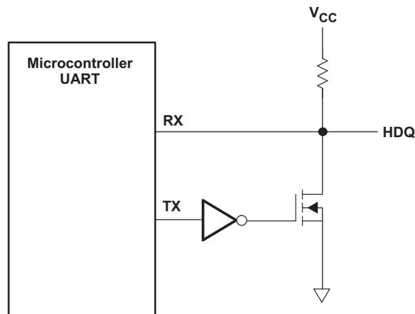
**Figure 5. HDQ Communication Using UART Without Open-Drain Output**
