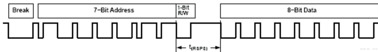
**Figure 1. Typical HDQ Read Cycle**
