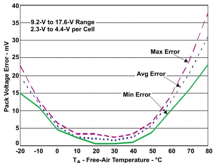
Figure 1. Pack Voltage Error vs Temperature
