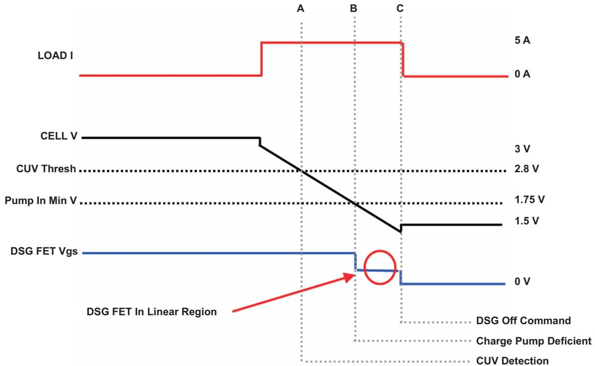
**Figure 4. Abnormal Cell Undervoltage Protection**
