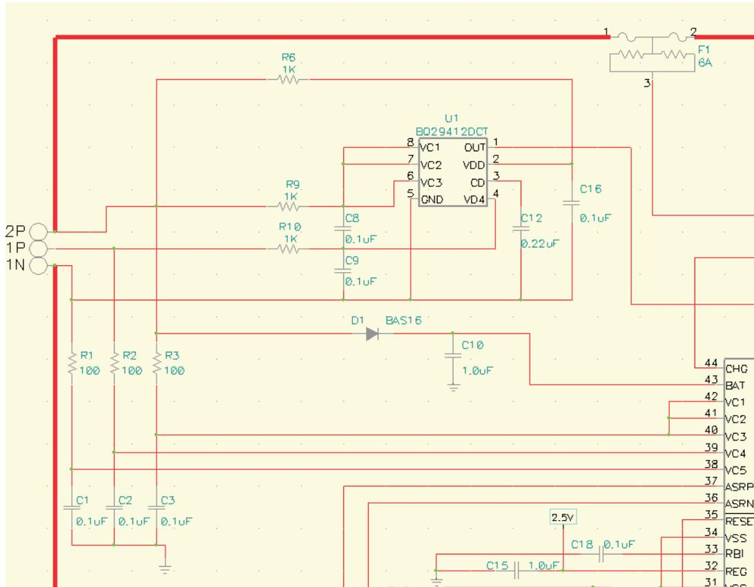
**Figure 1. 2-Series Cell Design Has VC1, VC2 and VC3 Pins Shorted on 2<sup>nd</sup> Voltage Protector and Fuel Gauge Battery Inputs.**
