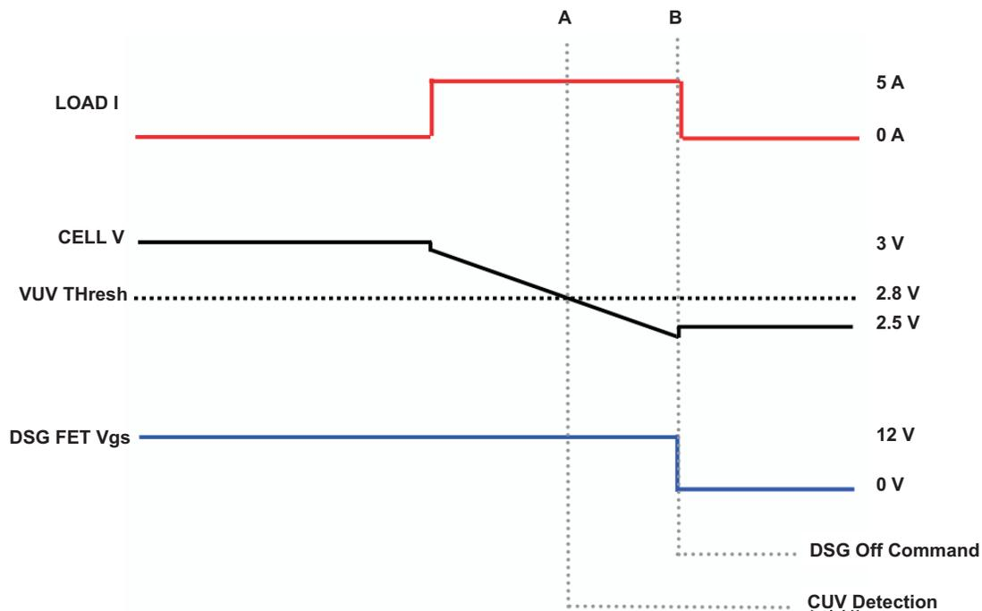
Figure 3. Normal Cell Undervoltage Protection
