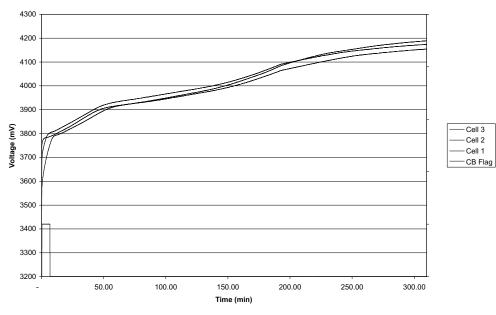
Cell Imbalance Tolerance - CB Min = 50 mV, CB Window = 100 mV
