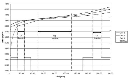
Figure 7. Cell Balancing Controlled in End Regions by CB Window
