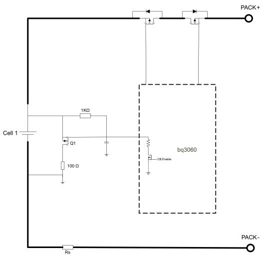
Figure 5. Cell Balancing Circuit
