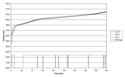
Figure 10. Cell Balancing with Low Imbalance Tolerance and Firmware Algorithm Infrequently Updated
