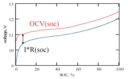
Figure 1. OCV and Voltage Under Load Profiles
