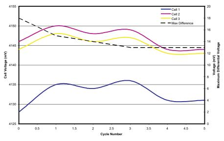
Figure 12. End of Charge Voltages of the Three Cells in Terms of the Cycle Number
