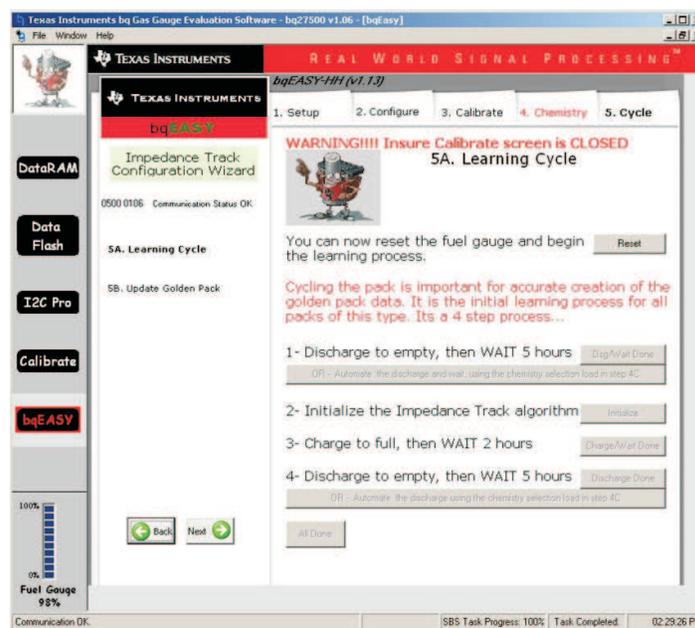
**Figure 6. bqEASY™ Semi-Automatic Cycle**
