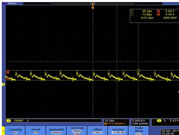
Full load ripple at 115V input CH1:100mV/div
