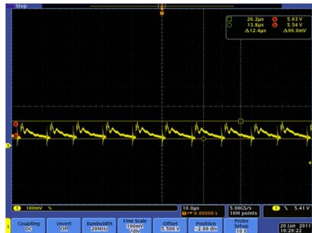
Full load ripple at 230V input CH1:100mV/div
