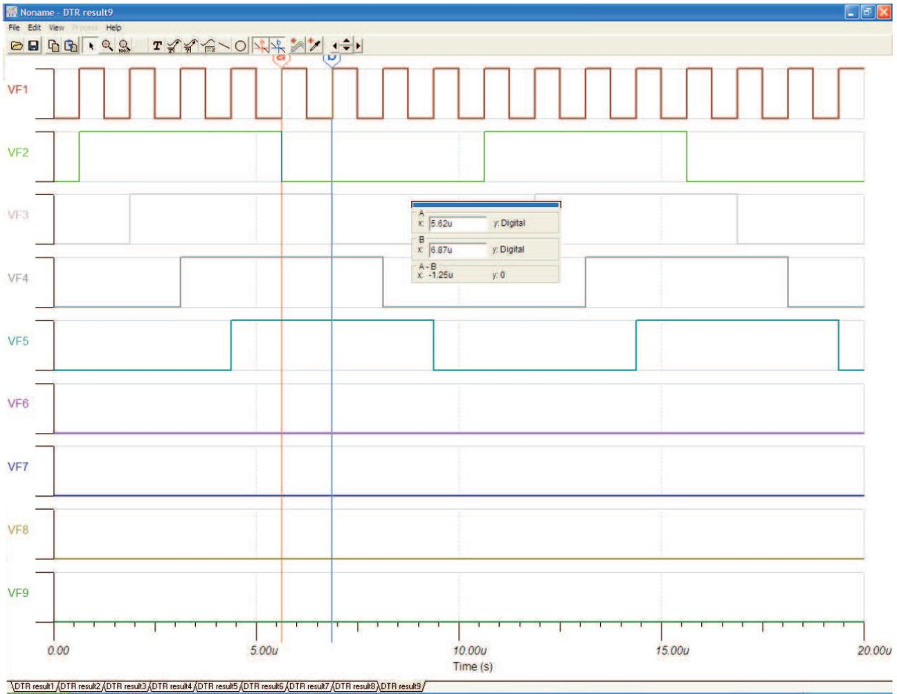
Figure 10. Waveforms of Dual, Four-Bit, Shift-Register Circuit
