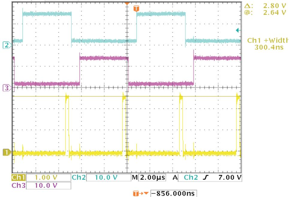
Ch. 1: Input to SYNC pin of slave UCC28950 (originating from function generator)
