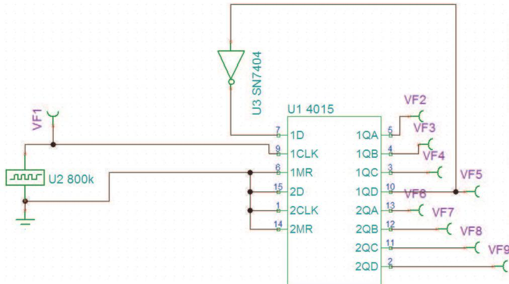
**Figure 9. Four-Bit Shift-Register to Generate Four, Phase-shifted SYNC Signals From a Single Clock Source**
