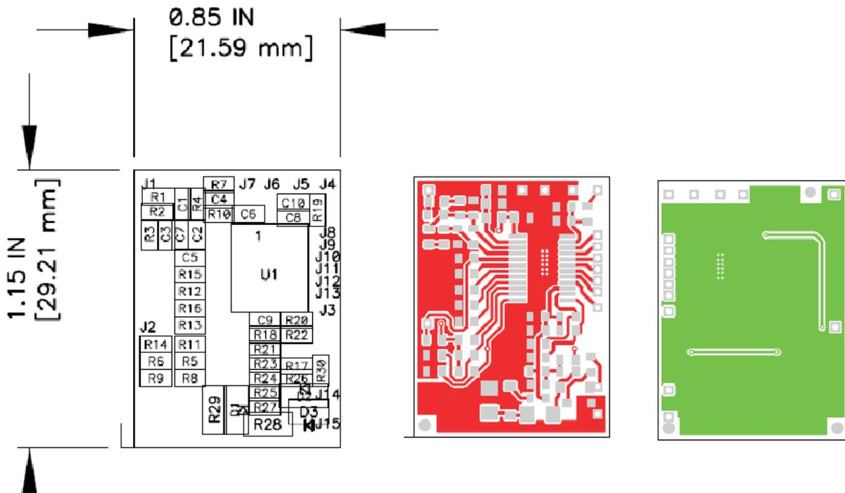
Figure 14. UCC28950 Small Control Card Layout and Assembly
