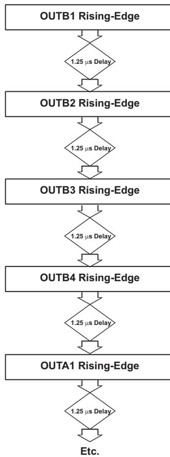
**Figure 4. Output Signals Rising-Edge Timing Flow**
