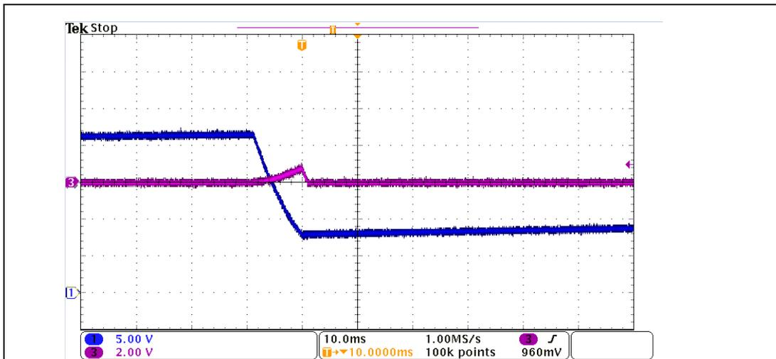
Figure 5. UCC28700 Start-up Waveform with  $C_{DD} = 4.7 \mu\text{F}$ ,  $R_{CS} = 2.05 \Omega$
