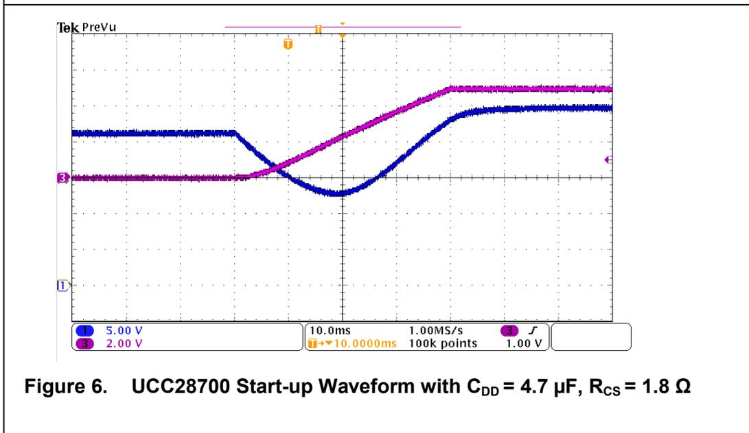
Figure 6. UCC28700 Start-up Waveform with  $C_{DD} = 4.7 \mu\text{F}$ ,  $R_{CS} = 1.8 \Omega$
