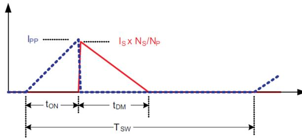
**Figure 3. Transformer Current**
