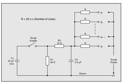
Figure 2. 10/700 µs Surge Generator as Defined in Figure A.3-1 of ITU-T K.44 Standard
