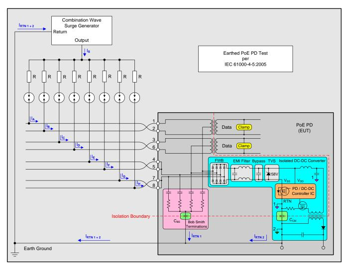
Figure 4. Example of Surge Current Paths Through an Earthed PD Application
