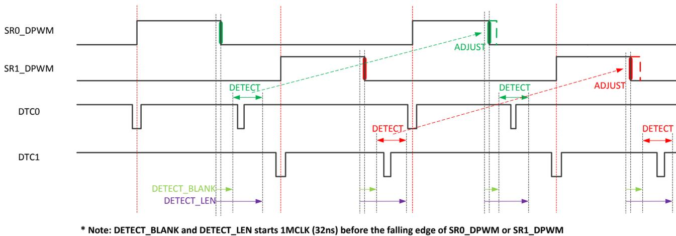
Figure 12. Timing Diagram of the DTC Interface
