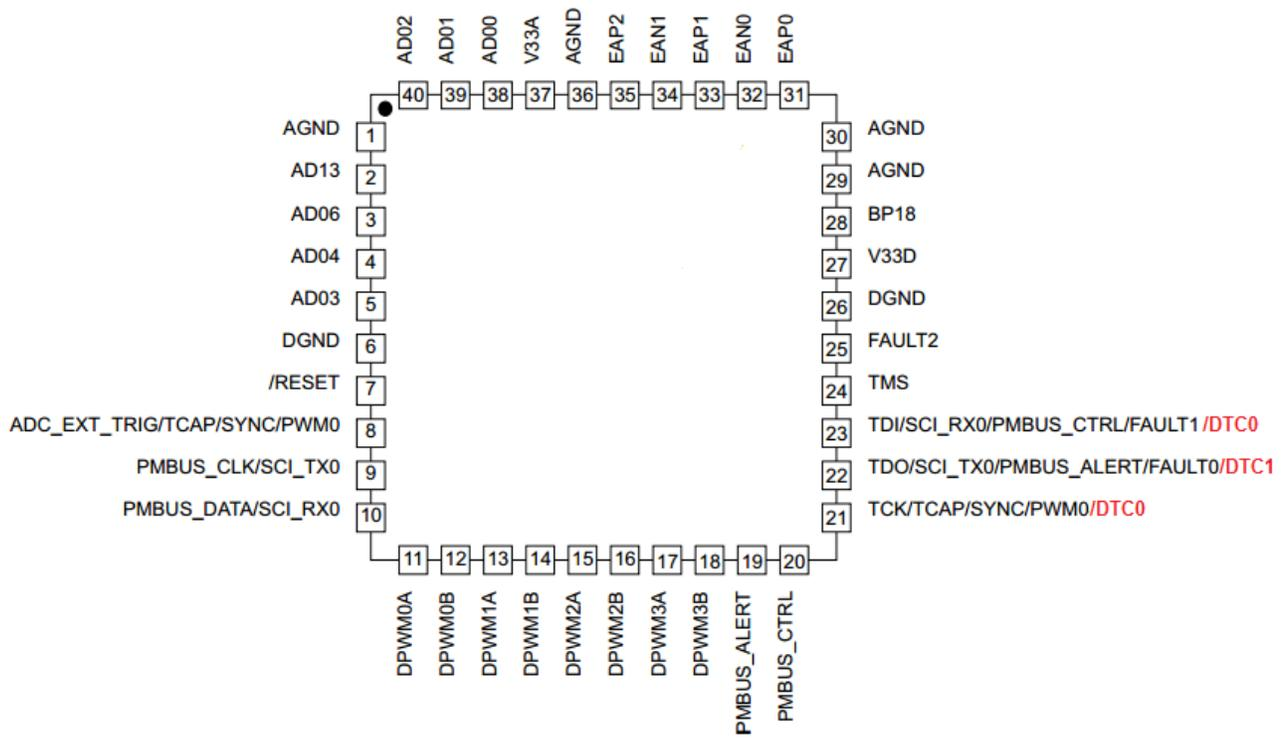
Figure 7. UCD3138A RMH Package Pin Out
