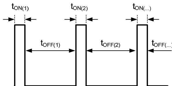
**Figure 2 - Ideal Modulator Output Pulse Train**
