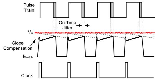
**Figure 12 - Peak Current Mode Control Real Modulator Waveforms**
