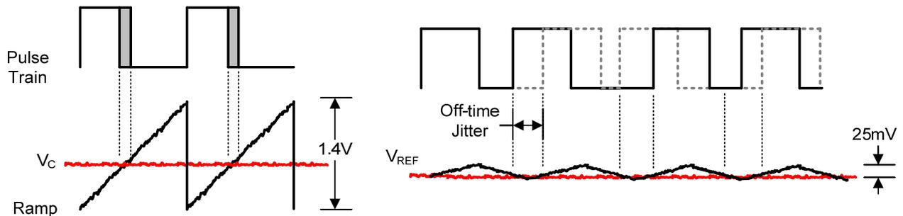
**Figure 23 - Noise Margin Comparison: Voltage Mode vs. DCAP**
