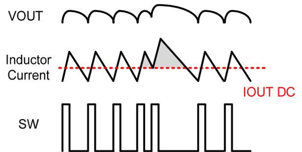
**Figure 25 - Jitter Response (DCAP)**
