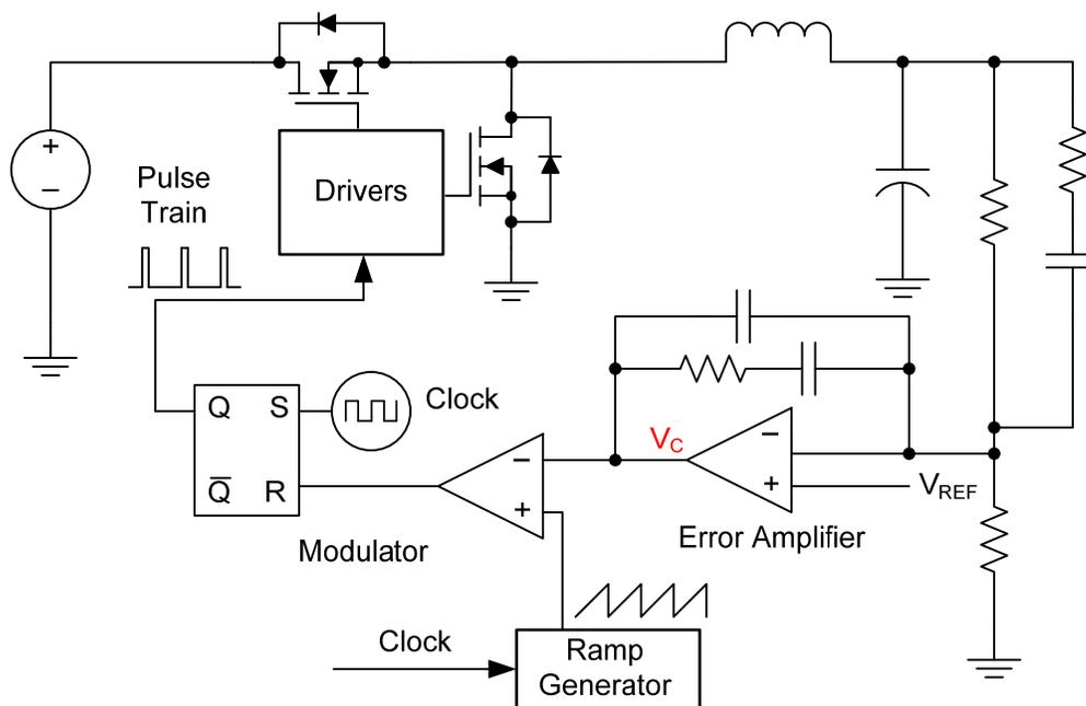
**Figure 6 - Voltage Mode Synchronous Buck Converter**
