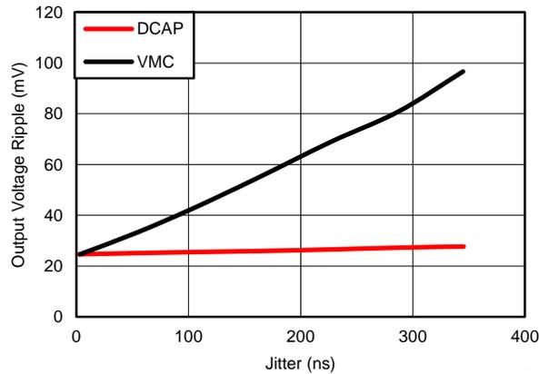
**Figure 21 - Simulation Result: Output Ripple vs. Jitter**
