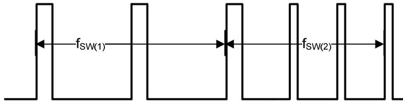
Figure 5 - Frequency Jitter
