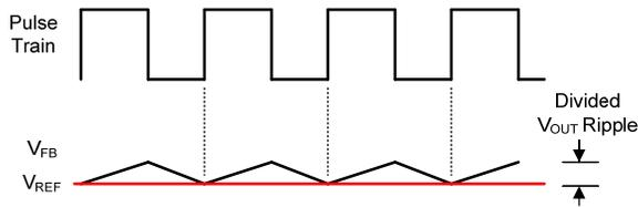
**Figure 15 - DCAP Ideal Modulator Waveforms**
