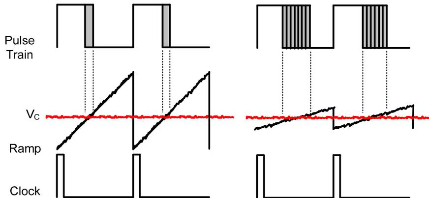
**Figure 9 - VM Modulator Noise Margin vs. Ramp Slope**
