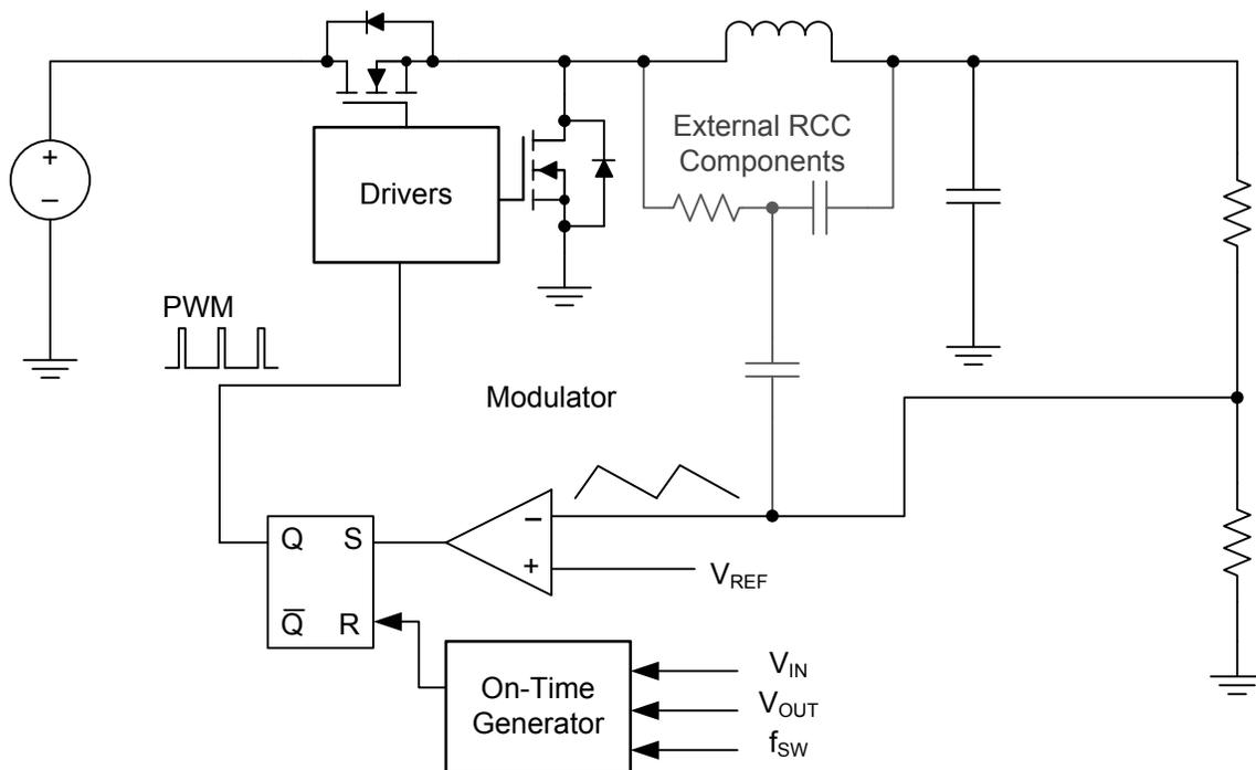
**Figure 18 - DCAP Control with External RC Ramp**
