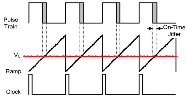
**Figure 8 - Real Modulator Waveforms**
