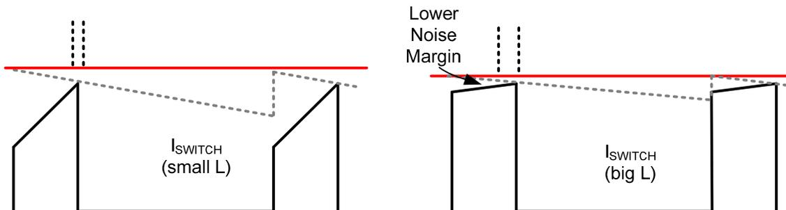
**Figure 13 - Peak Current Mode Control Inductor Slope Dependence**
