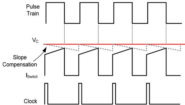
**Figure 11 - Peak Current Mode Control Ideal Modulator Waveforms**
