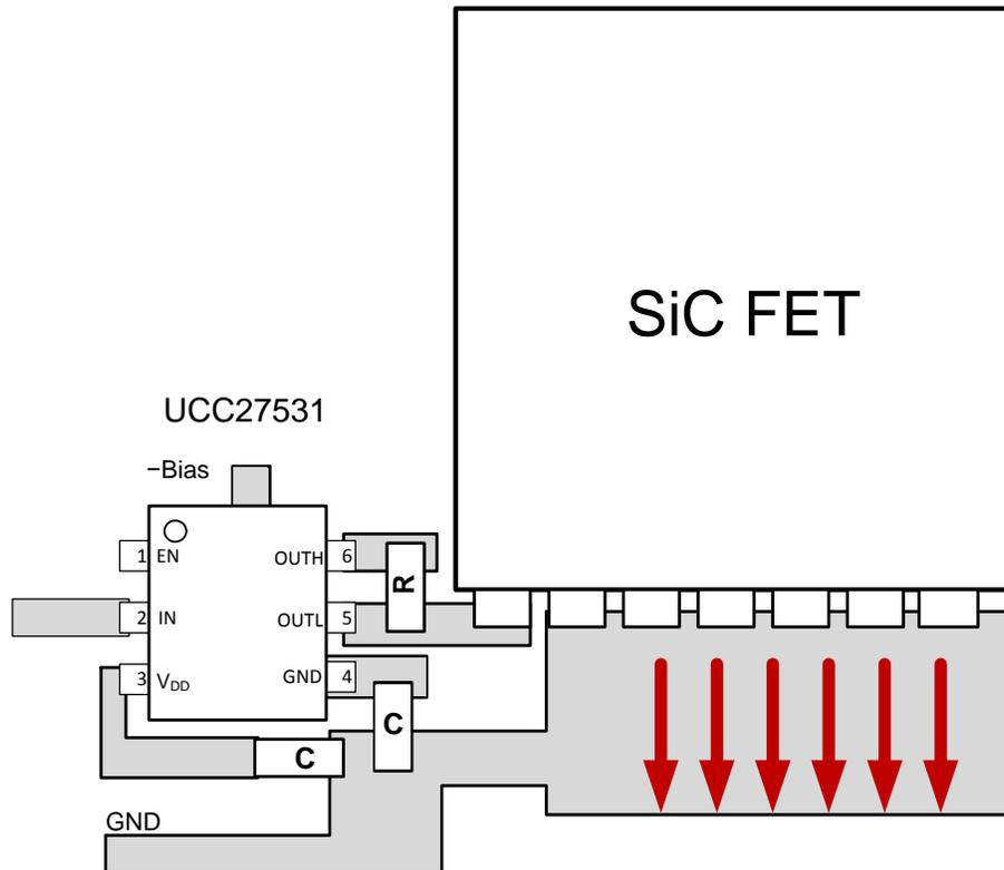
Figure 12. Driver and MOSFET Layout
