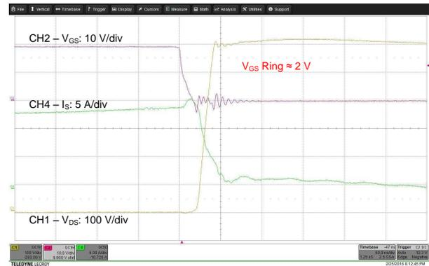
Figure 9.  $V_{DS}$ ,  $V_{GS}$ ,  $I_S$  Turnoff, No Negative Drive
