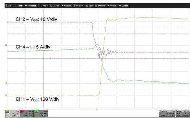
Figure 8.  $V_{DS}$ ,  $V_{GS}$ ,  $I_D$  Turnoff Transition
