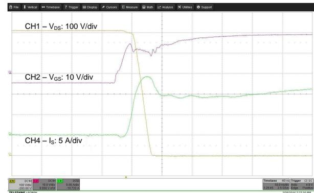
Figure 7.  $V_{DS}$ ,  $V_{GS}$ ,  $I_S$  Turnon Transition
