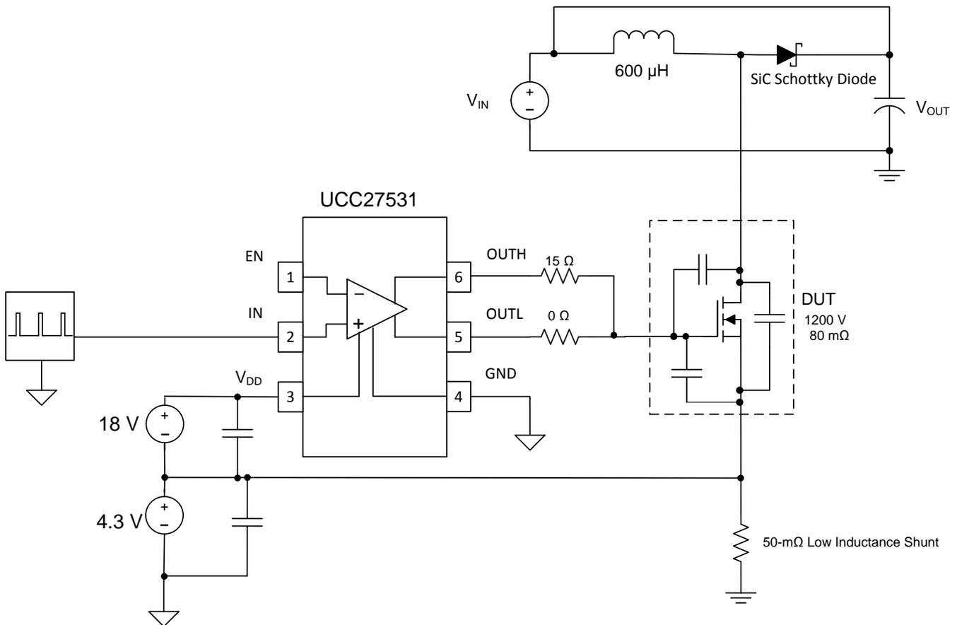
Figure 5. UCC27531 SiC MOSFET Demonstration Circuit Diagram
