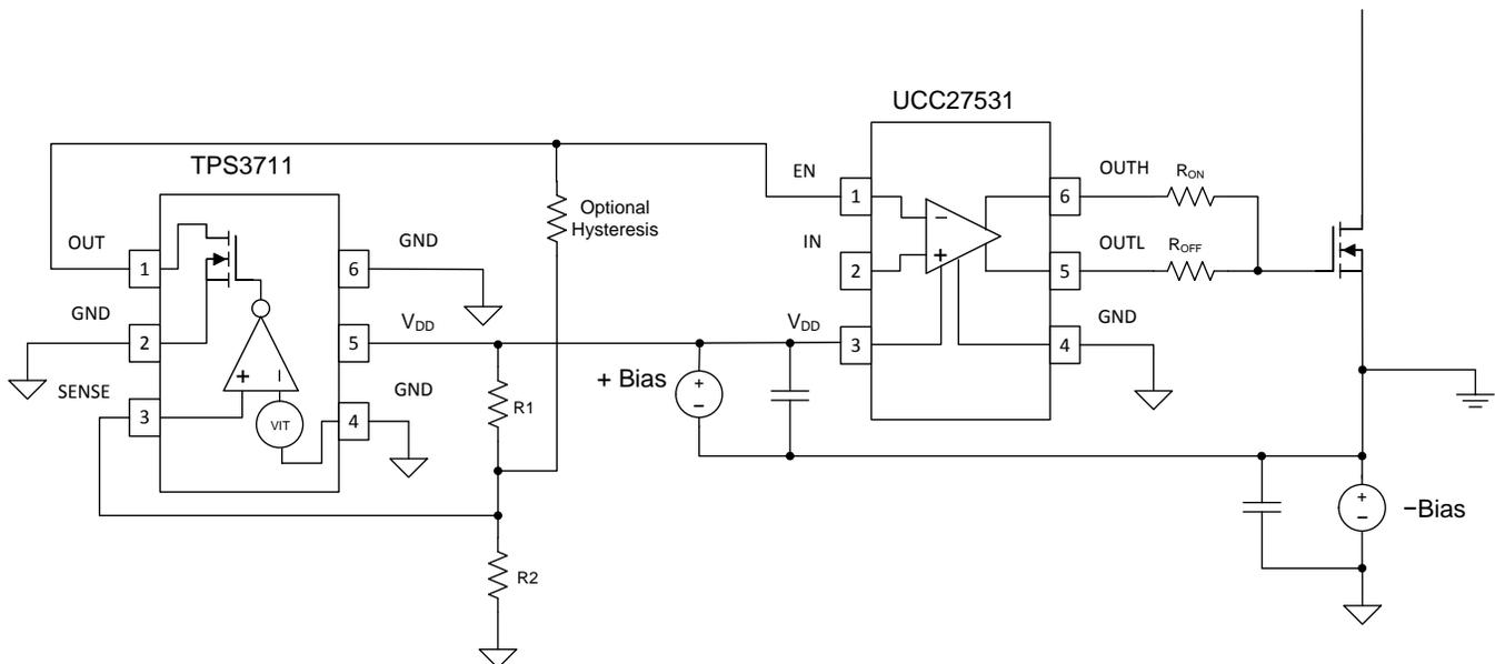
**Figure 11. TPS3711 to Program UCC27531 UVLO Thresholds**
