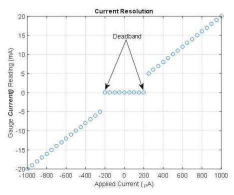
Figure 1. Gauge Reported Current vs Applied Current
