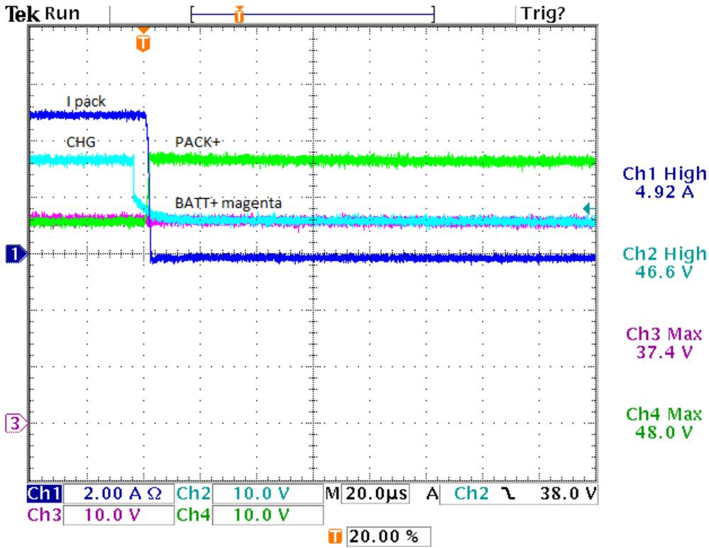
Figure 5. Charge FET Switching With Normal Circuit
