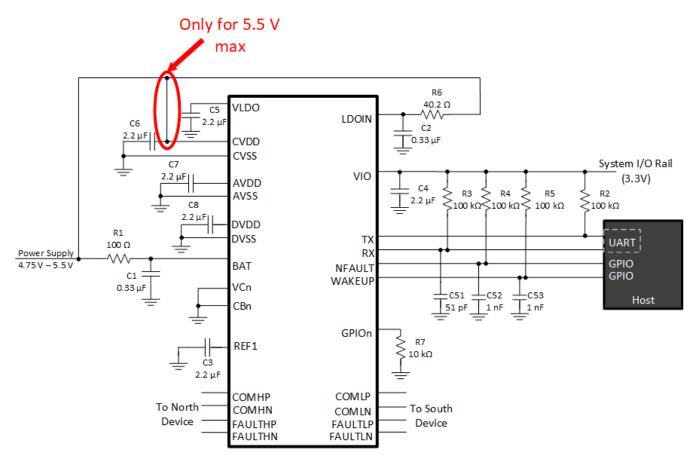
Figure 17. Bridge Device Schematic for 4.75 V to 5.5 V
