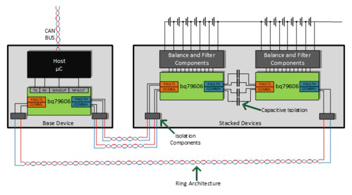
Figure 14. Using BQ79606A-Q1 as Bridge Device Block Diagram
