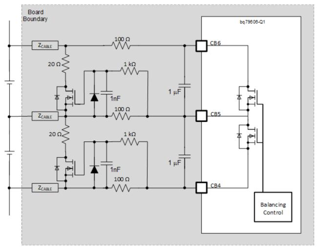
Figure 8. External FET Cell Balancing
