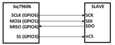
Figure 13. Example SPI Master Connections
