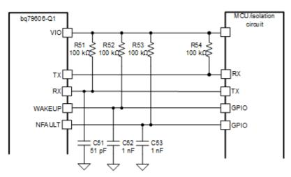
Figure 18. Connecting WAKEUP and Communication for Bottom Device
