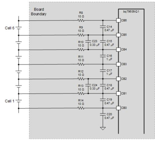
Figure 6. Cell Balancing
