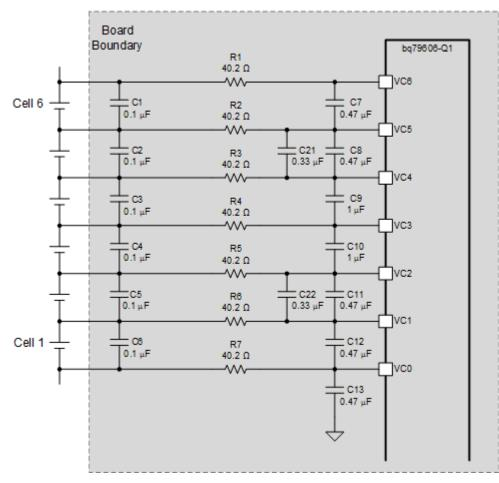
Figure 5. Cell Voltage Monitoring
