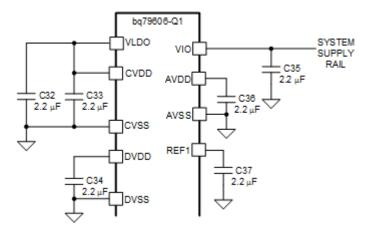
Figure 2. Regulator Connection for Base Device
