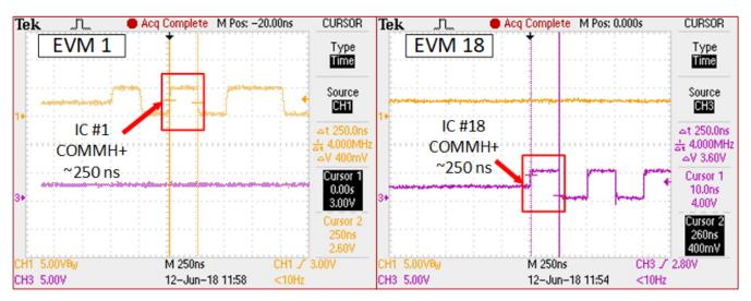
Figure 23. Re-Clocking Bit Compression Example
