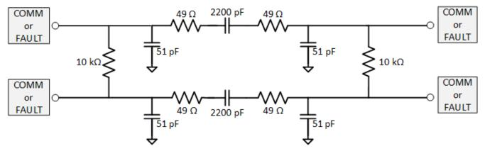
Figure 20. Noise Isolation for Devices on Same PCB
