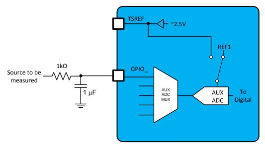
Figure 12. GPIO Absolute Voltage Measurement
