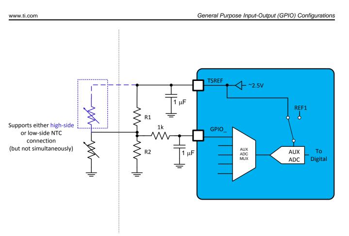
Figure 11. GPIO Ratiometric Measurement
