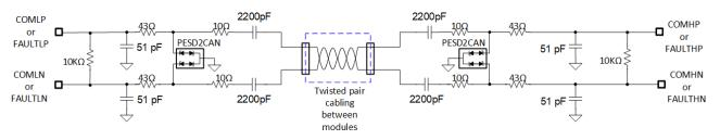
A. Components Required for Capacitive Coupled Daisy Chain with Cabling < 2m
