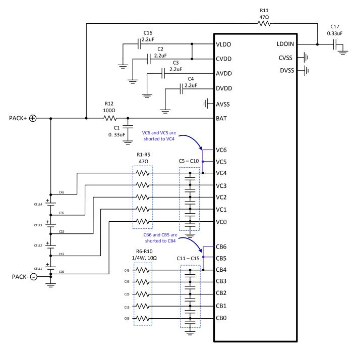
Figure 10. Connecting Fewer than 6 Cells
