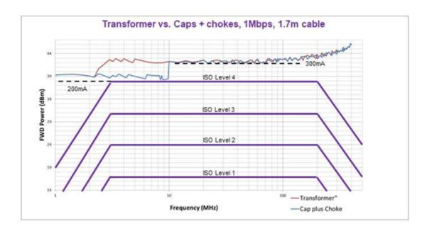
Figure 31. Transformer vs Cap & Choke BCI Plot
