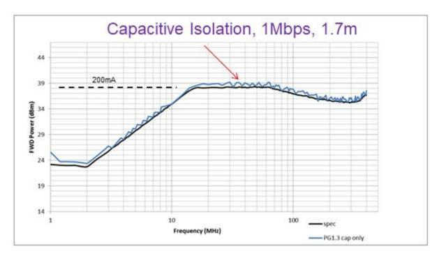
Figure 29. Capacitive Isolation BCI Plot
