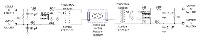
Figure 33. Transformer Isolation Schematic
