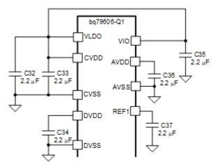
Figure 3. Regulator Connection for Stack Device
