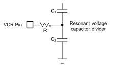
Figure 6. Additional Circuitry on VCR Pin
