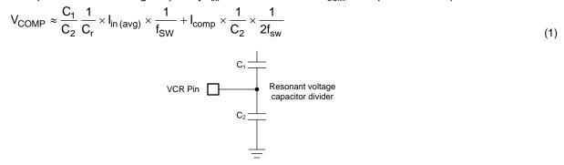
Figure 4. VCR Pin Capacitor Divider
