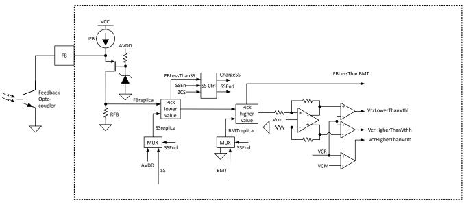
Figure 7. Feedback Chain Block Diagram
