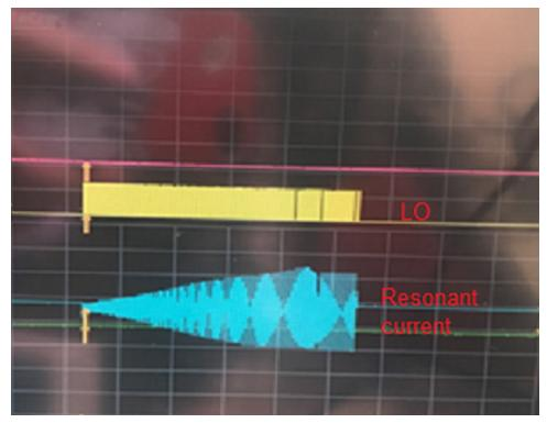
Figure 11. Test Waveform With Soft Burst on Circuit
