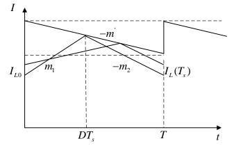
Figure 3. Inductor Current and Slope Compensation Waveform
