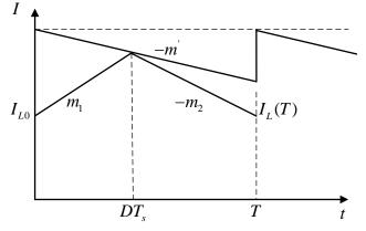
Figure 2. Inductor Current and Slope Compensation Waveform
