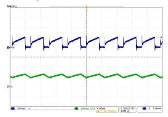
Figure 5. UCC2897A 18-V Input (Blue is the V<sub>cs</sub>, Green is the Inductor Current)
