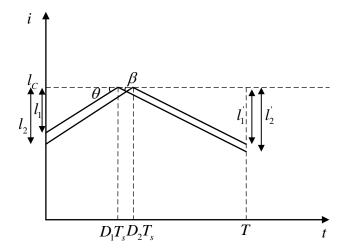
Figure 1. Inductor Current Waveform With Disturbance
